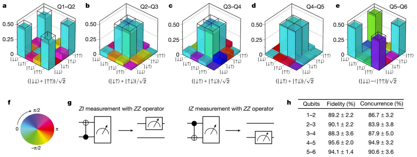
**Fig. 4 | Bell state tomography.** **a–e**, Measured two-qubit density matrices for qubits Q1–Q2 (**a**), Q2–Q3 (**b**), Q3–Q4 (**c**), Q4–Q5 (**d**) and Q5–Q6 (**e**), after removal of SPAM errors (see Supplementary Information for the uncorrected density matrices). The target Bell states are indicated and outlined with the wireframes. **f**, Colour wheel with phase information for the density matrices presented in **a–e**. **g**, Quantum circuits used for converting parity readout (ZZ)
