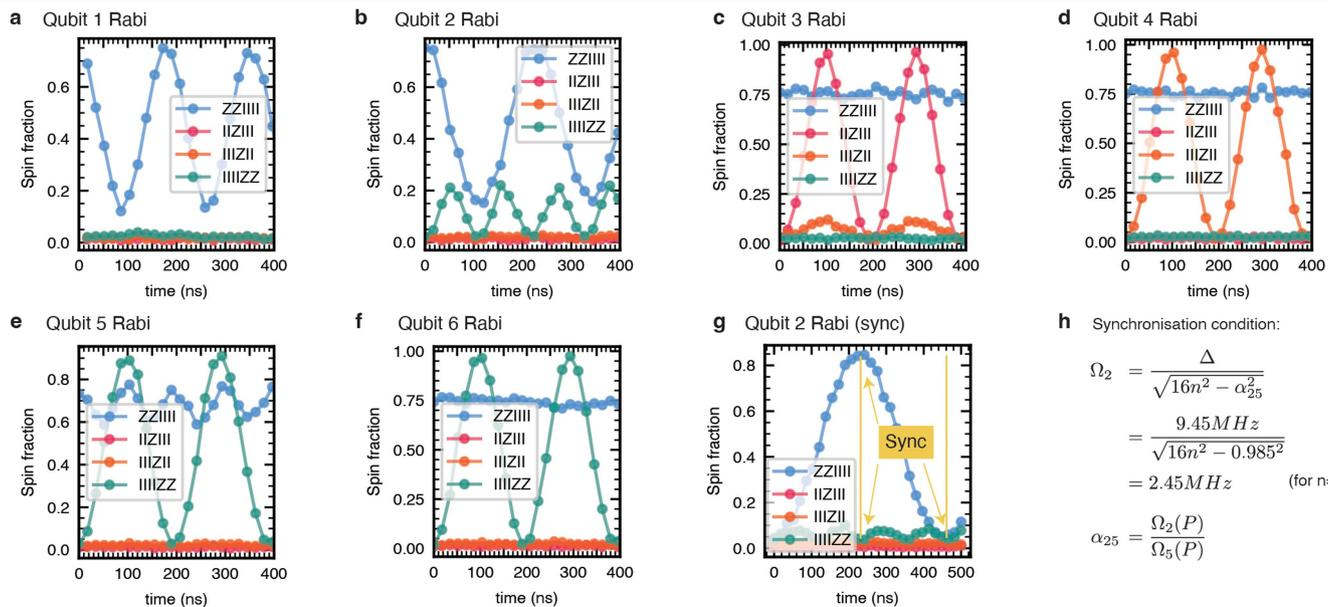
**Extended Data Fig. 5 | Crosstalk. a-f**, In this experiment all qubits are initialized. We observed the presence of crosstalk by measuring the expectation values of the native observables on the sample. **a-e**, Rabi oscillations executed on different qubits in each panel. Panels b, c and e display coherent oscillations of nominally idle qubits, which are a clear indication of crosstalk at the chosen Rabi frequencies. Qubits Q1 and Q2 show flipped
