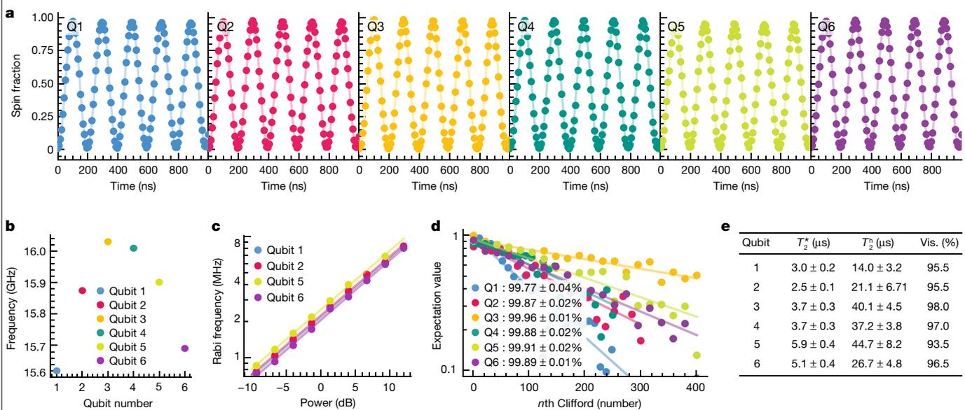
**Fig. 2 | Single-qubit gate characterization.** **a**, Rabi oscillations for every qubit, taken sequentially. The spin fraction refers to the spin-up fraction for qubits Q2–Q5 and to the spin-down fraction for qubits Q1 and Q6. The drive amplitudes were adjusted in order to obtain uniform Rabi frequencies of 5 MHz. **b**, Qubit frequency for each of the six qubits. **c**, Rabi frequency of each qubit as a function
