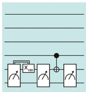
**Extended Data Fig. 2 | Full quantum circuits. a.** This circuit was used to produce the data presented in Fig. 5c. The different background colors indicate the different parts of the sequence (yellow – initialization, green – manipulation (including the tomography pulses), blue – readout). The
