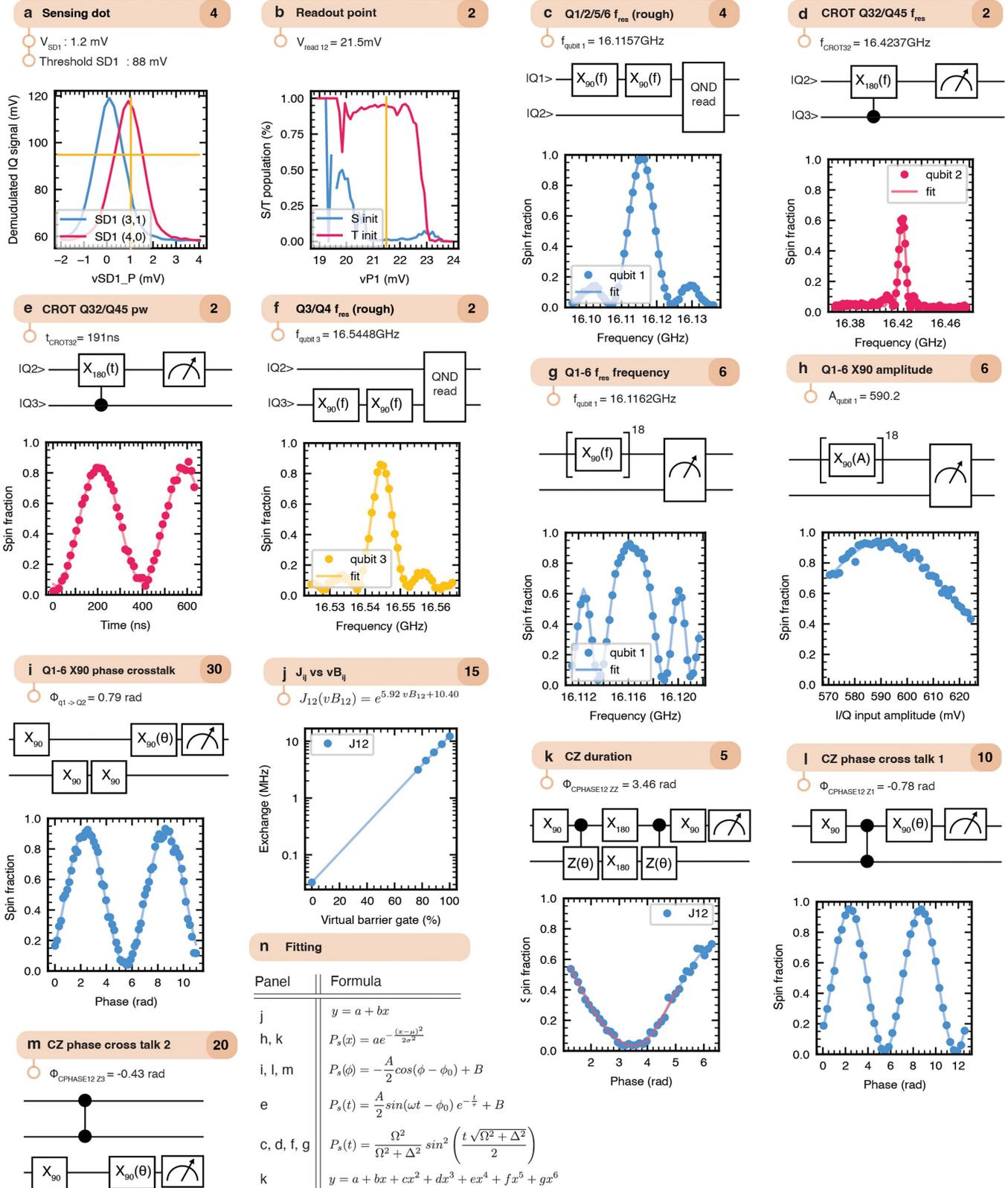
**Extended Data Fig. 4 | Calibrations.** a–m Each panel shows a typical experimental dataset obtained in one of the calibration routines for the relevant experimental parameters. Every panel indicates in the header the calibration name and the corresponding number of calibration parameters.
