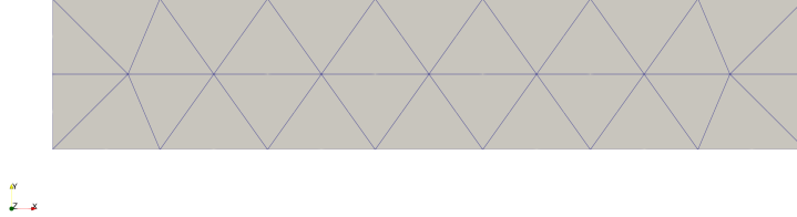
(b) Mesh used in the post-buckling problem.
