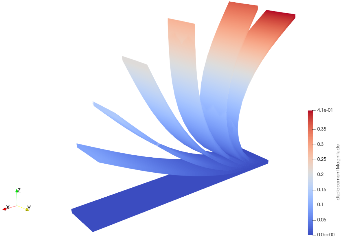
Figure 4.6: Several configurations of the post-buckled beam with eight layers.
