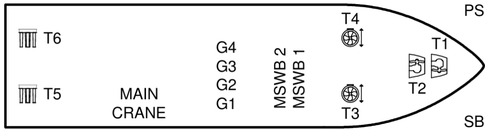
Figure 7.1: Vessel Load-Layout of the Reference Vessel S [16]
