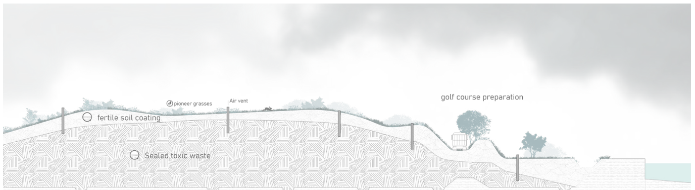
Figure 79: Zoom in on section of waste collection hub (current situation)
