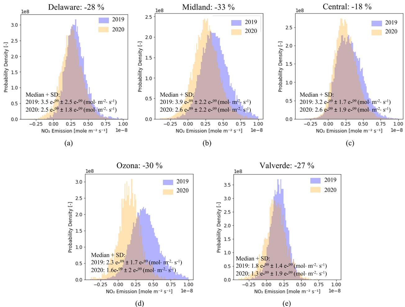
**Figure 5.** Histograms of the NO<sub>2</sub> emissions for the most productive sub-basins (a, b, and c) and the less productive (d and e) in the Permian basin during the period April-May in 2019 and 2020. The percentages in the plot title are related to the reduction of NO<sub>2</sub> emissions between 2019 and 2020 (SD: Standard deviation).
