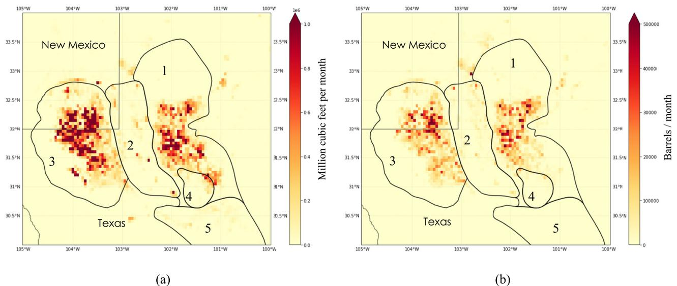
**Figure 2.** Monthly average of gas (a) and oil (b) production distribution in the Permian basin in 2020. The numbers are related to the different sub-basins of the Permian: 1-Midland, 2-Central, 3-Delaware, 4-Ozona Arc, and 5-Valverde.
