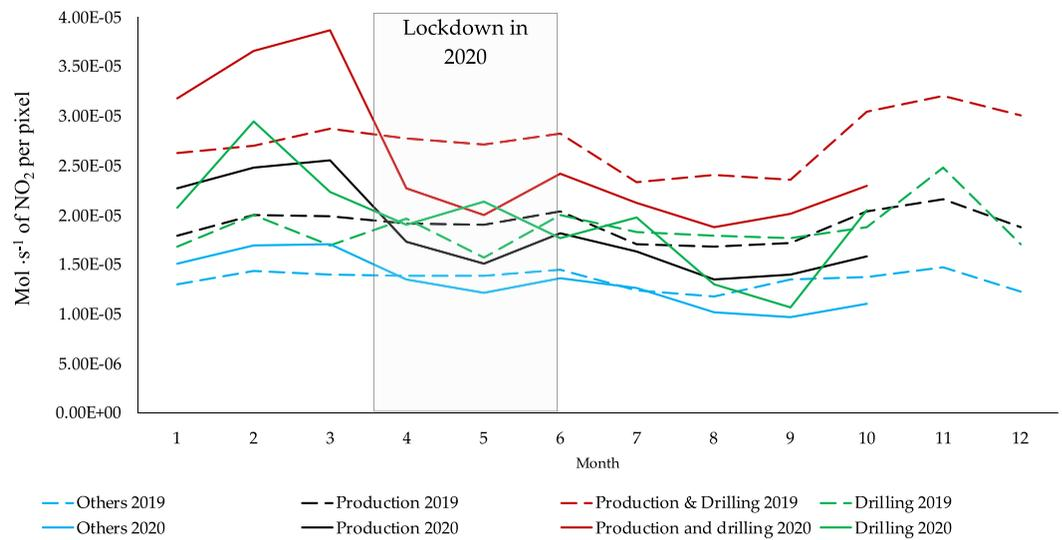
**Figure 6.** Normalized NO<sub>2</sub> emission for each month in areas with only production, production and drilling, drilling, and other activities not related to the O&G. NO<sub>2</sub> emissions were normalized by the number of pixels attributed to each activity on the entire Permian basin.
