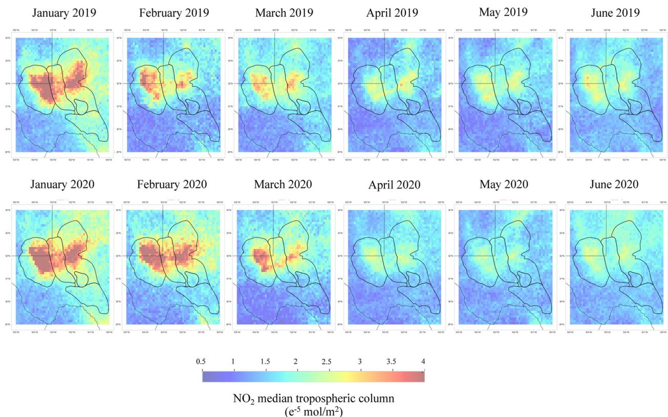
**Figure 3.** Time series of median nitrogen dioxide tropospheric column from January to June 2019 and 2020 in the Permian basin.
