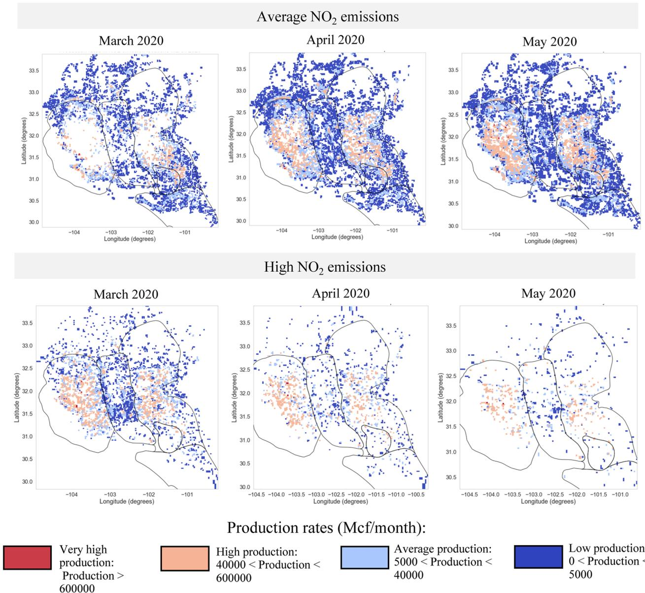
**Figure 7.** NO<sub>2</sub> high emissions ( $4.3 \text{ e}^{-9} \text{ mol}\cdot\text{s}^{-1}\cdot\text{m}^{-2} < \text{NO}_2 \text{ emissions} < 9.3\text{e}^{-9} \text{ mol}\cdot\text{s}^{-1}\cdot\text{m}^{-2}$ ) (Bottom) and average emissions ( $3.5 \text{ e}^{-10} \text{ mol}\cdot\text{s}^{-1}\cdot\text{m}^{-2} \leq \text{emissions} \leq 4.3 \text{ e}^{-9} \text{ mol}\cdot\text{s}^{-1}\cdot\text{m}^{-2}$ ) (Top) related to gas production rates in the Permian basin from March to May 2020.
