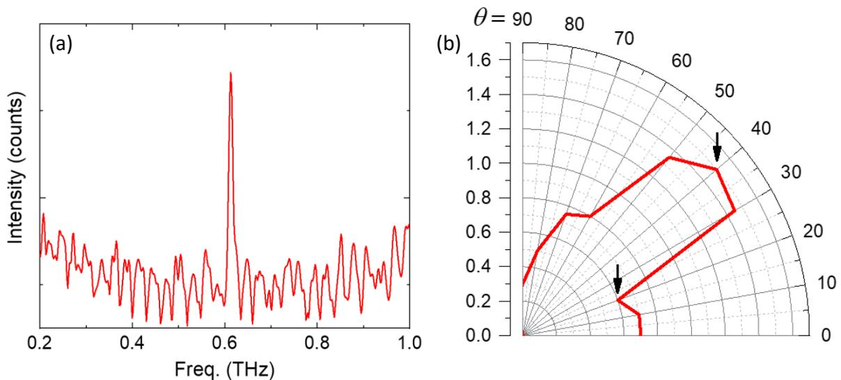
Figure 1. (a) The radiation spectra from an isosceles triangular mesa measured by the FT-IR spectrometer at the current  $I = 0.7$  mA and voltage  $V = 0.9$  V of the outermost IVC, at temperature  $T = 30$  K. (b) The angular  $\theta$  dependence of the radiation intensity (in one measured experimental run), obtained in the  $yz$  plane. The arrows indicate the first minimum and absolute maximum for  $\theta > 0$ .
