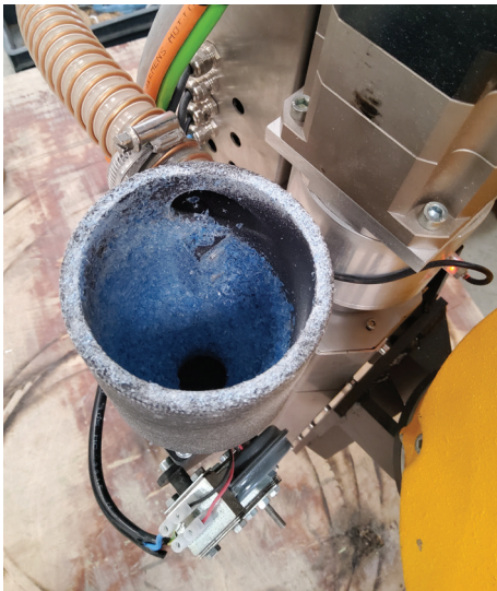
Figure 8: Small, statically charged particles sticking to the sensors and hopper walls.
