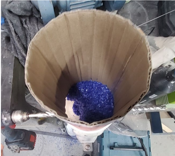
Test 8: Round opening, vertical, with concrete drill: Extreme tunnelling, but hopper is emptied entirely. Stream is less consistent compared to horizontal setup.
