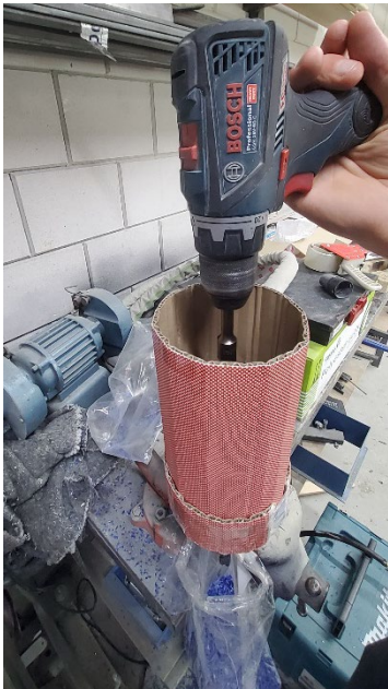
Test 9: Round opening, vertical, with concrete drill with steel wire flow aid: Steel wire stirs nicely, but in a filled hopper it is too weak. The wire winds itself around the drill.
