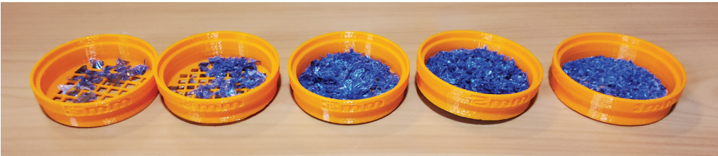
Figure 25: Flake size distribution from a 3mm granulator (Left to right: 5 mm, 4 mm, 3 mm, 2 mm and 1 mm, square hole size).
