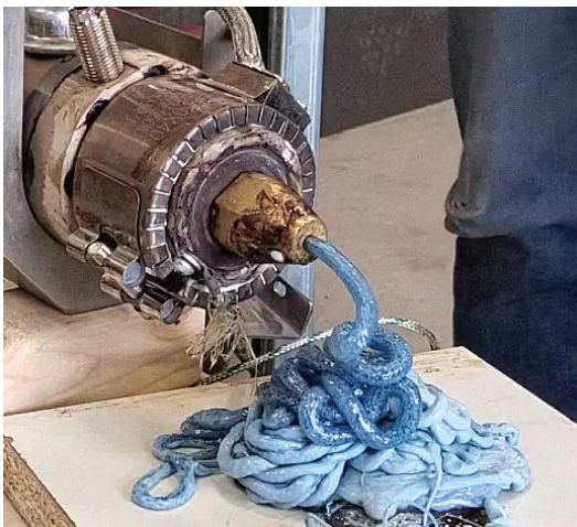
Figure 9: Bubbles in output and opaque PET: the result of hydrolysis when processing undried PET.
