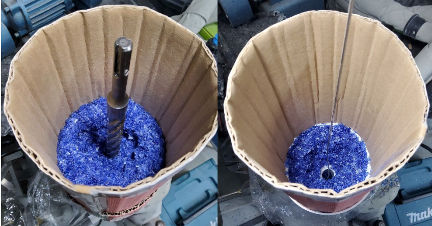
Test 6: Round opening, vertical, with air channels: Blowing air through the hopper does not work. Possibly due to the air channels being too small or to little pressure.
