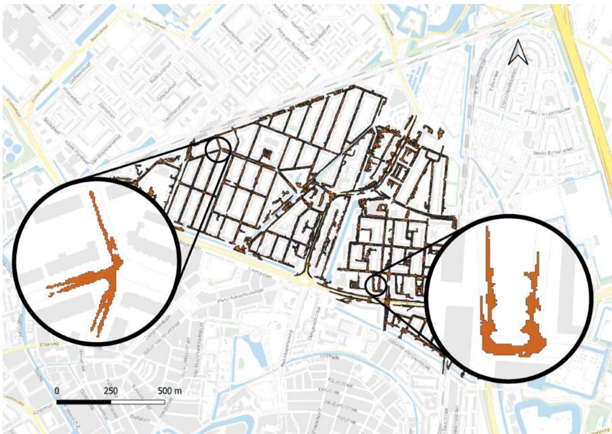
Figure H.1: Flooded area at manholes in case of sewer hydraulic failure in Tuindorp
