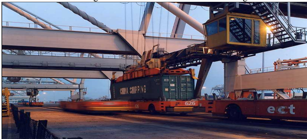
Figure 9.8: AGV's loaded/unloaded between crane legs
