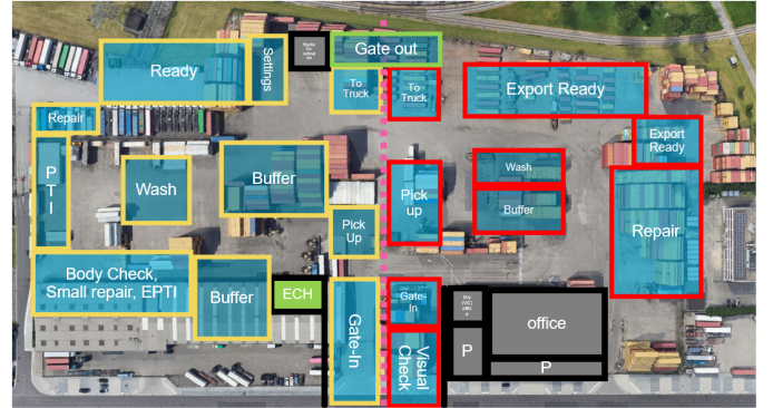
Fig. 7. Schematic overview of setting 6 layout ECD
