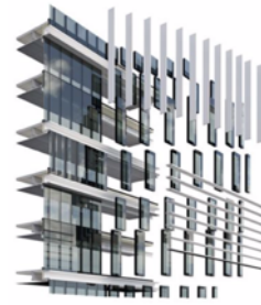
Figure 39 – Drawing of a facade which is designed for disassembly
