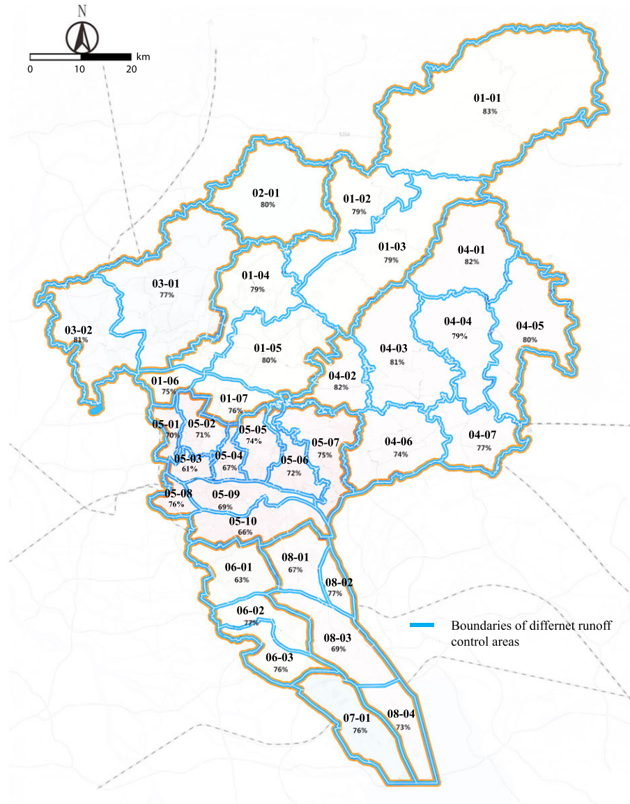
FIG. 7.5 Runoff control regulatory codes for flood resilience / Source: Author, based on Guangzhou Sponge City Plan 2010-2030 (Guangzhou Government 2017)
