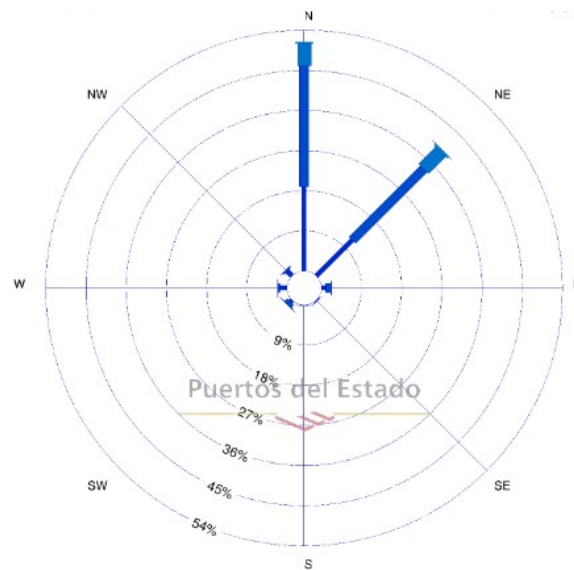
Figure 3: Wave direction distribution near Gran Canaria. Wave rose for the wind at the Gran Canaria location, wave direction is plotted in regard to the probability of occurrence [1].
