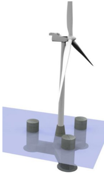
Figure 6: IEA 15 mounted on the semi-submersible floater [1].
