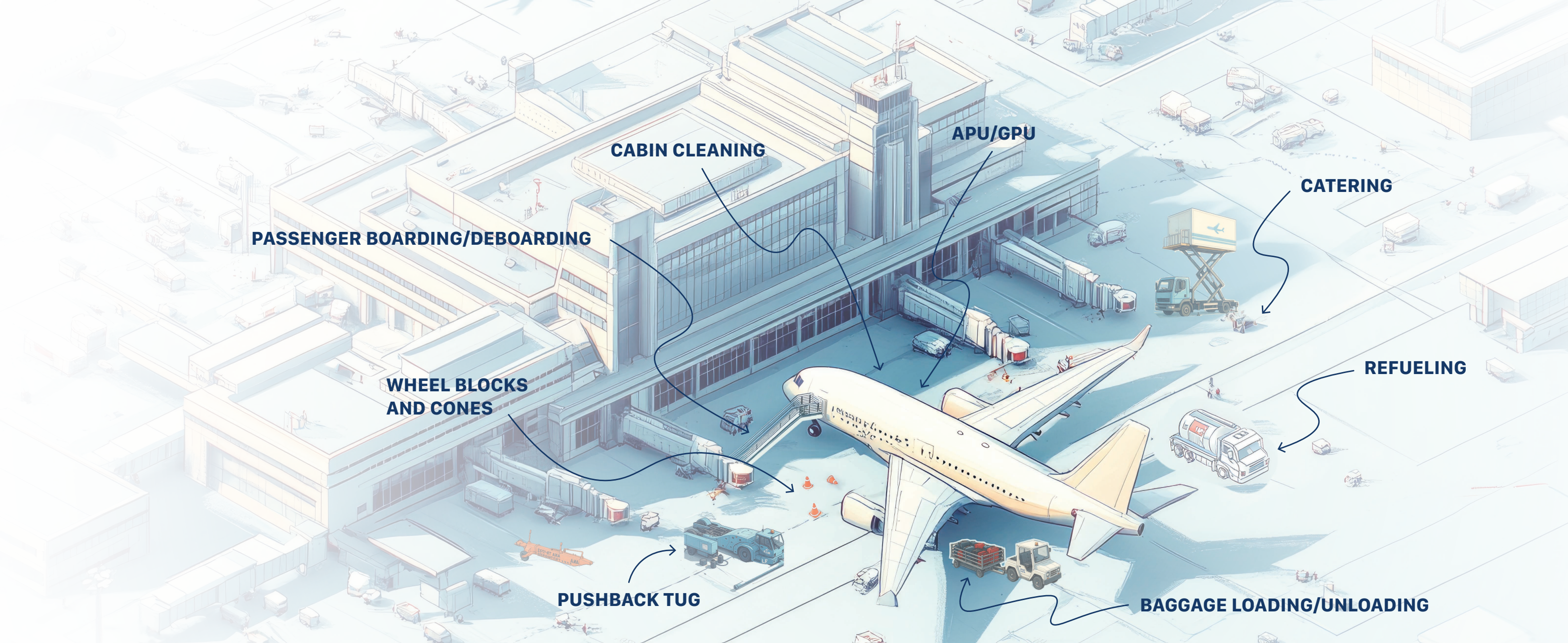
A visual representation of some of the equipment involved in a long-haul turnaround, and their placement airside.
