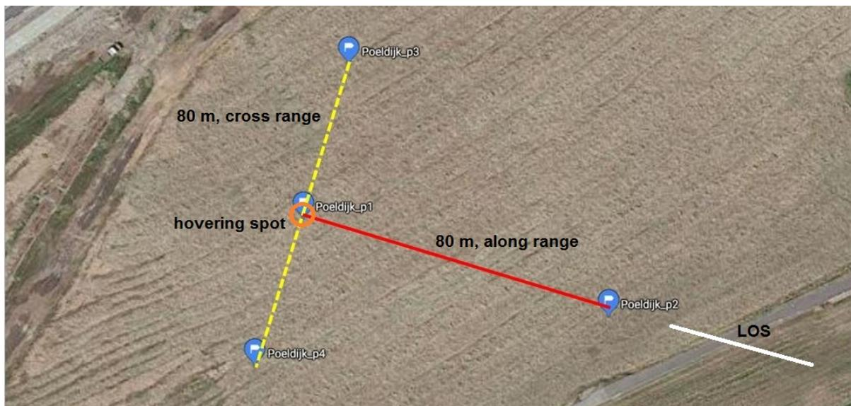
Figure 5.1: Motion paths of the drones in the experiment field: (a) Orange spot – Hovering, (b) Red line – Along range maneuvering, (c) Yellow dashed line – Cross range maneuvering
