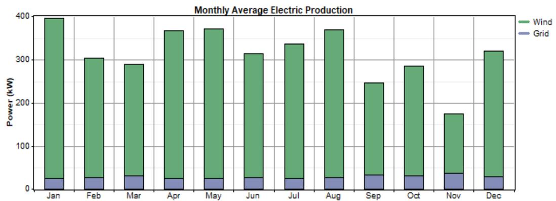
Figure 5. 11 Monthly power generation by DC micro-grid components case-II.
