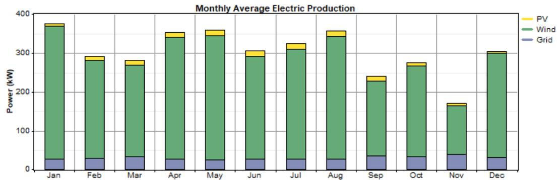
Figure 5. 2 Monthly power generation by AC micro-grid components case-I.
