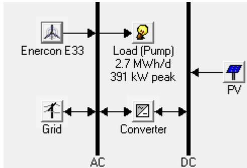
Figure 5. 22 Block diagram hybrid AC/DC micro-grid 150% load Case-II.
