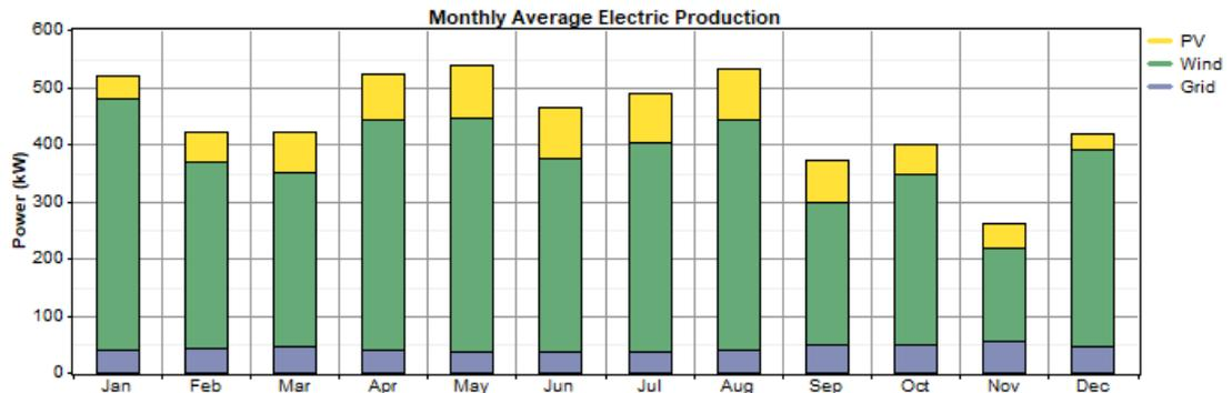
Figure 5. 20 Monthly power generation by hybrid AC/DC micro-grid components 150% load Case-I.
