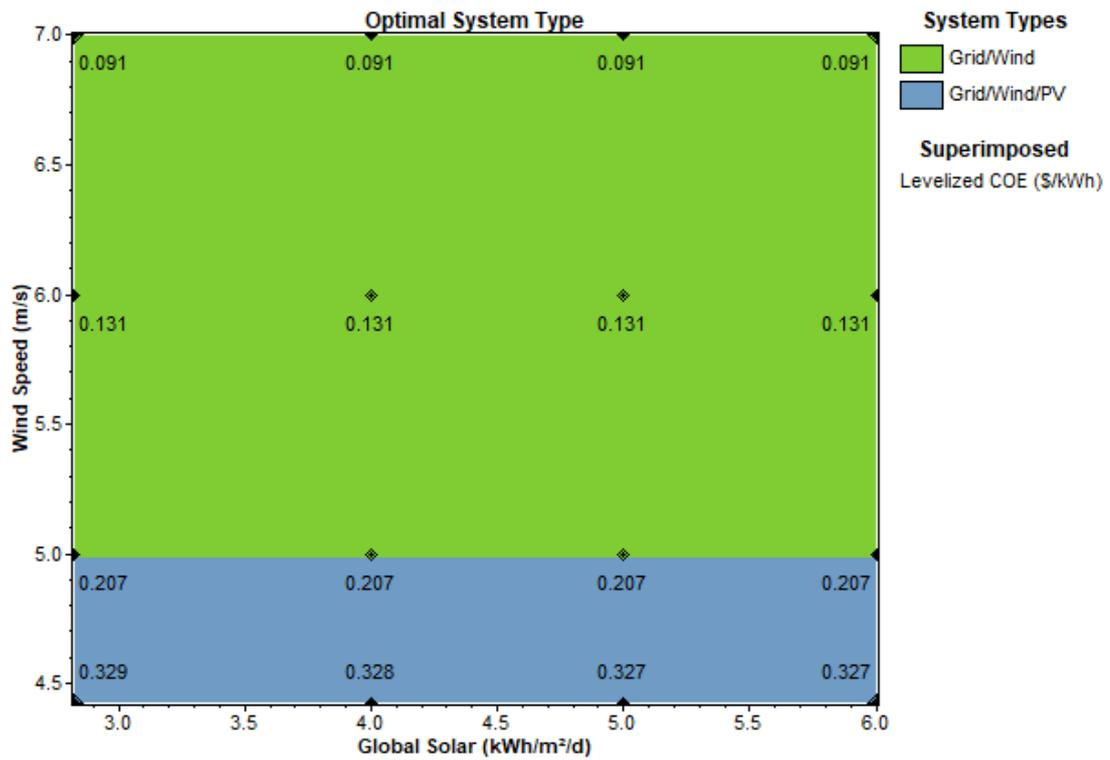
Figure 5. 3 Unit energy cost changes in case-I AC micro-grid.
