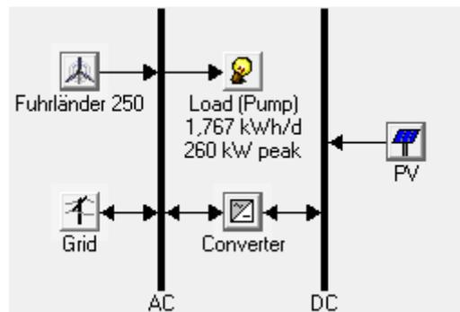
Figure 5. 13 Block diagram of hybrid AC/DC micro-grid case-I.
