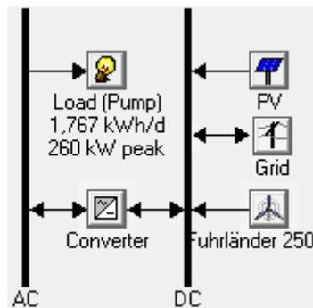
Figure 5. 7 Block diagram of DC micro-grid case-I.
