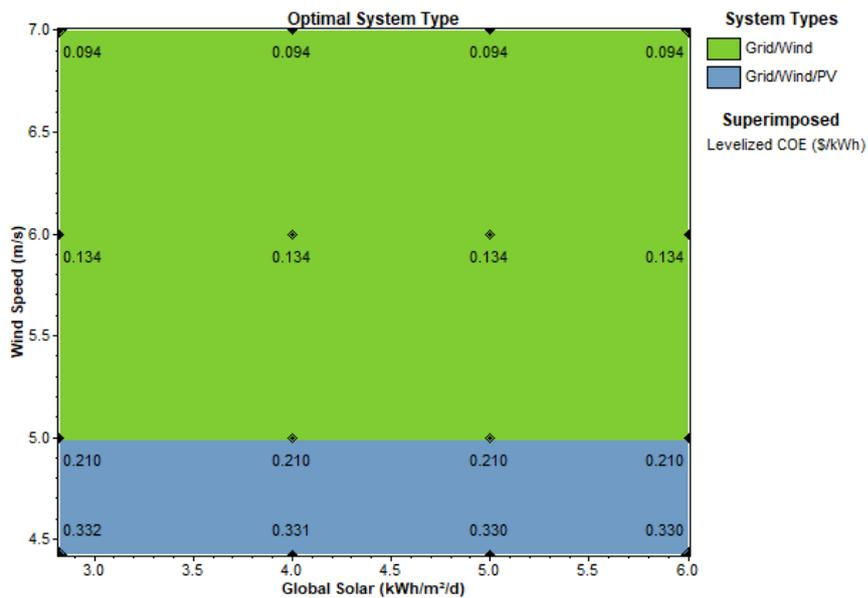
Figure 5. 9 Unit energy cost changes in case-I DC micro-grid.
