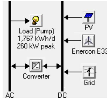
Figure 5. 10 Block diagram of DC micro-grid case-II.
