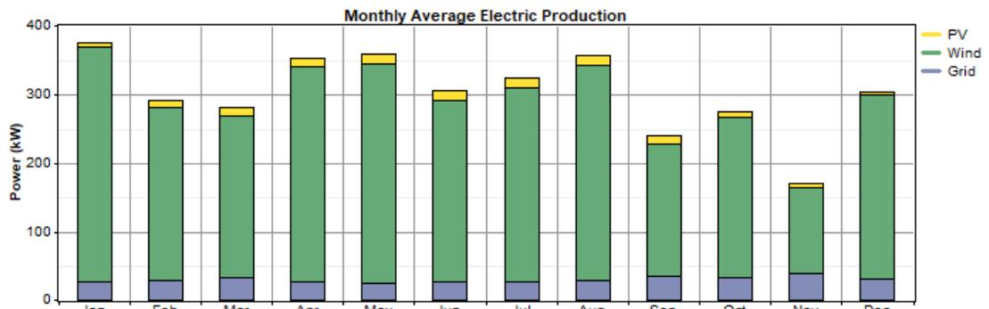
Figure 5. 14 Monthly power generation by hybrid AC/DC micro-grid components case-I.
