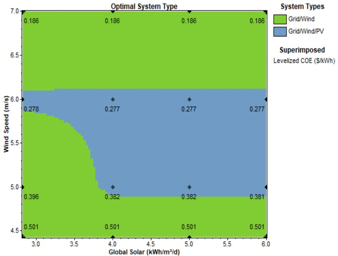
Figure 5. 18 Unit energy cost changes in case-II hybrid AC/DC micro-grid.
