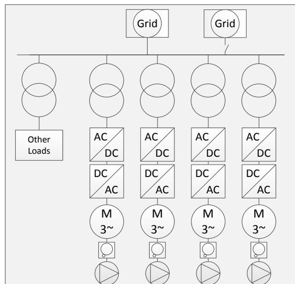
Figure 3. 1 Current System Components.
