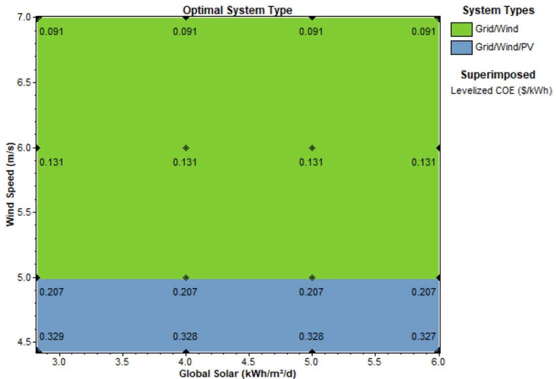
Figure 5. 15 Unit energy cost changes in case-I hybrid AC/DC micro-grid.
