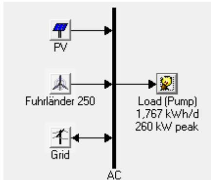
Figure 5. 1 Block diagram of AC micro-grid case-I.
