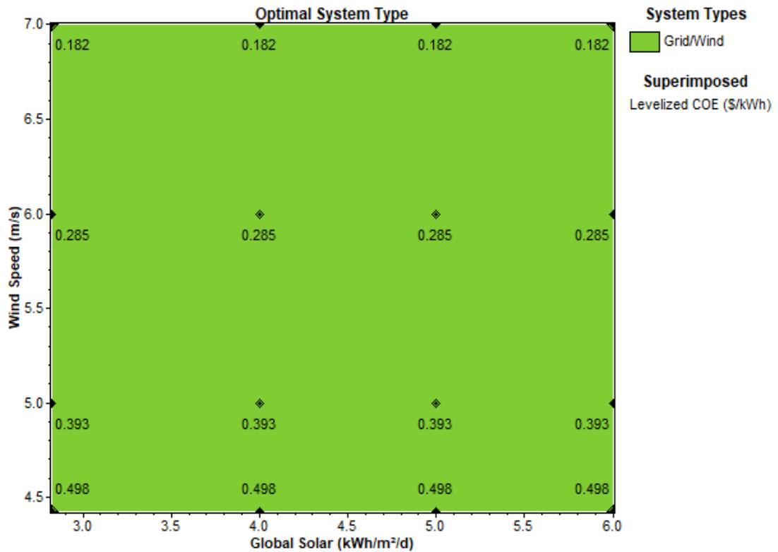
Figure 5. 12 Unit energy cost changes in case-II DC micro-grid
