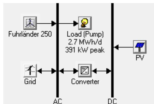
Figure 5. 19 Block diagram hybrid AC/DC micro-grid 150% load Case-I.
