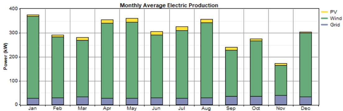
Figure 5. 8 Monthly power generation by DC micro-grid components case-I.
