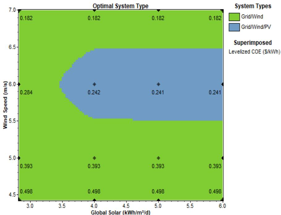
Figure 5. 6 Unit energy cost changes in case-II AC micro-grid.
