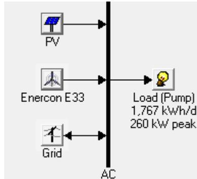
Figure 5. 4 Block diagram of AC micro-grid case-II.
