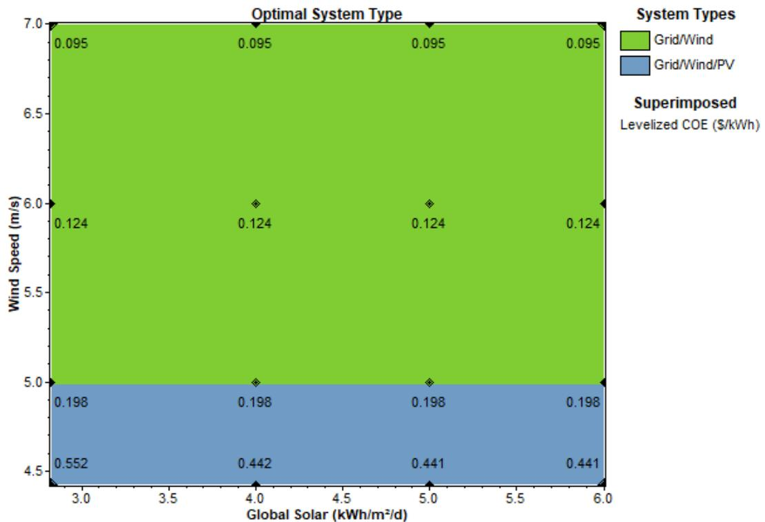
Figure 5. 21 Unit energy cost changes in hybrid AC/DC micro-grid 150% load Case-I.
