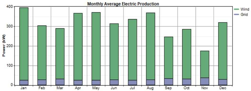
Figure 5. 5 Monthly power generation by AC micro-grid components case-II.
