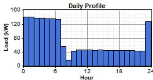
Figure 4. 4 Daily load profile of the pump.
