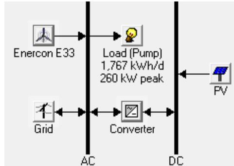
Figure 5. 16 Block diagram of AC-DC Hybrid micro-grid of Case-II.
