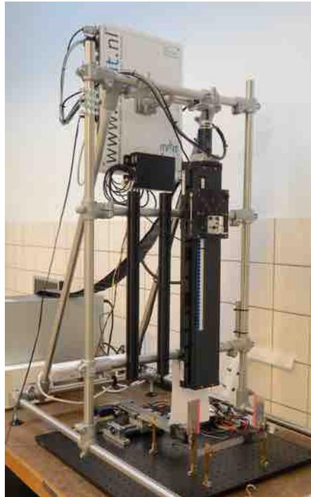
**Figure B.1:** Motorized stage used at the TU Delft to perform needle insertion experiments while insertion forces are measured with the ATI Nano 17.
