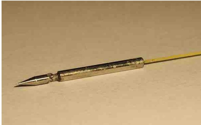
**Figure 4.7:** Prototype of the unmachined-quartz-column concept with needle tip.
