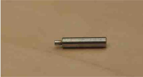
**Figure 5.3:** Tool used to position the quartz ferrule in the Invar stylet tube and determine the FPI cavity length.
