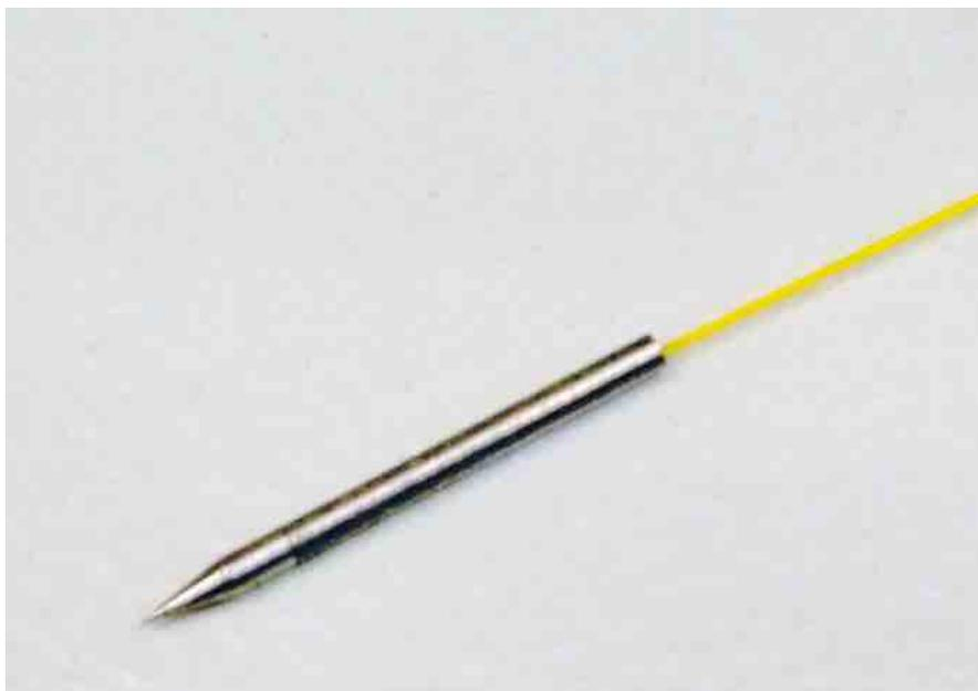
**Figure 5.2:** Assembled prototype of the stylet-tube concept.
