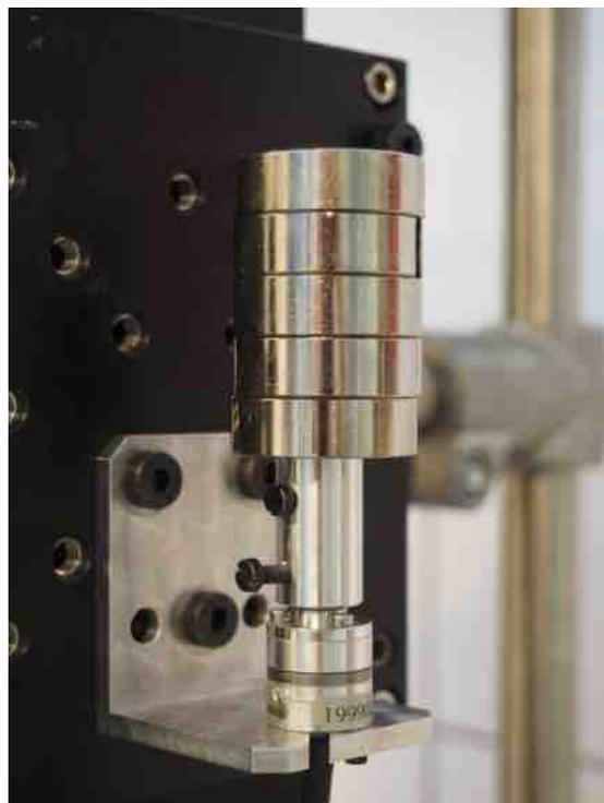
**Figure B.2:** Stack of weights on the ATI sensor to generate a well defined calibration force.
