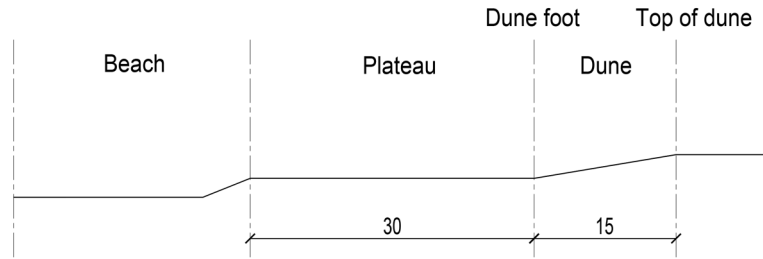
Figure 3.2: Typical coast cross-section showing the plateau and the dunes relatively to the beach. The dimensions of the plateau and the dunes are assumed to be constants and are in meter
