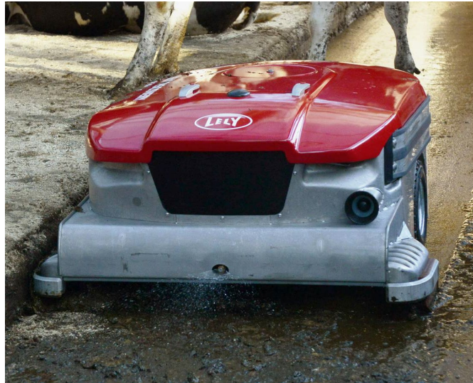
Figure 12 - Collector vacuuming manure.
