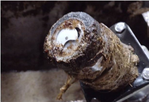
Figure 53 - Manure build-up on lens of sensor.
