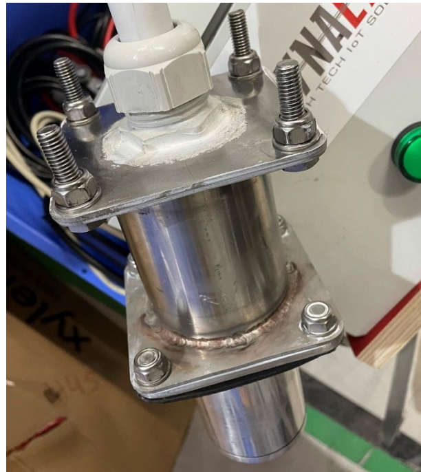
Figure 50 - Modified waterproof sensor head
