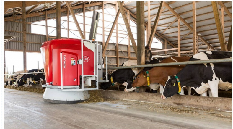
image / figure 2: Current Lely autonomous vehicle for feeding.
