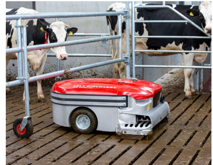
Figure 11 - The Collector drives in between the cows.
