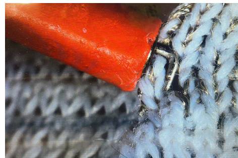
FIGURE 70: MICROSCOPE PHOTO OF ELECTRODE CONNECTION HOOK
