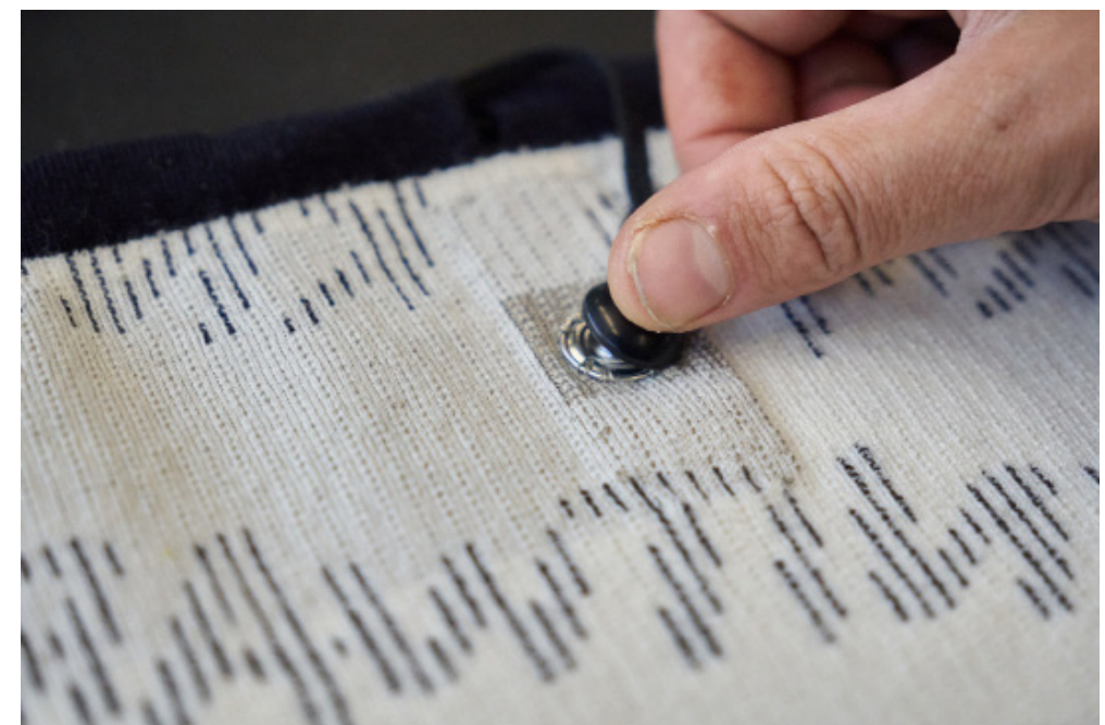
FIGURE 10: CLOSING THE BUTTON TO MAKE CONNECT THE BATTERY
