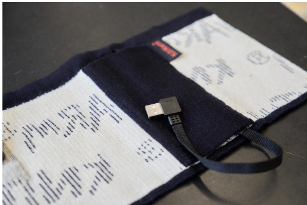
FIGURE 8: BATTERY CONNECTION OF KNITWARM SCARF
