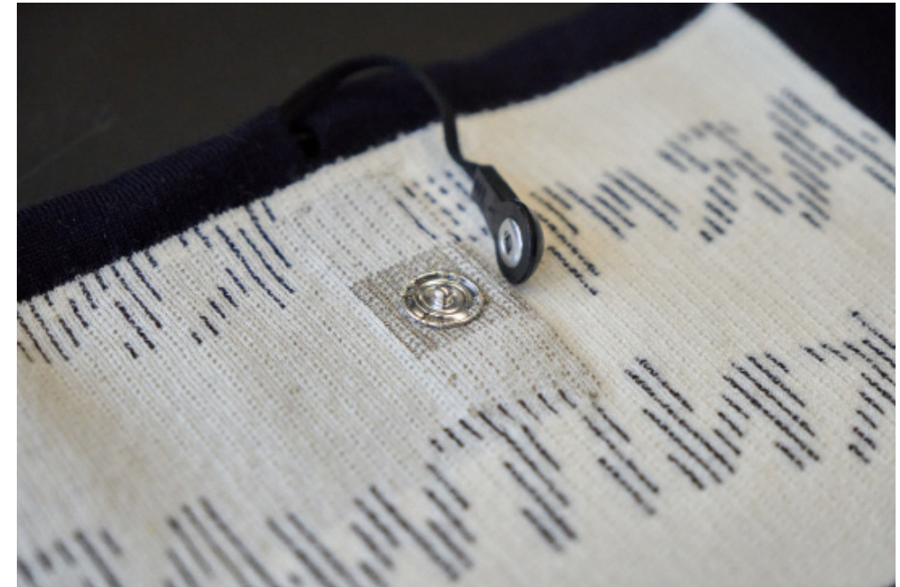
FIGURE 9: DETAIL OF KNITWARM SCARF: A BUTTON IS USED TO CONNECT THE BATTERY
