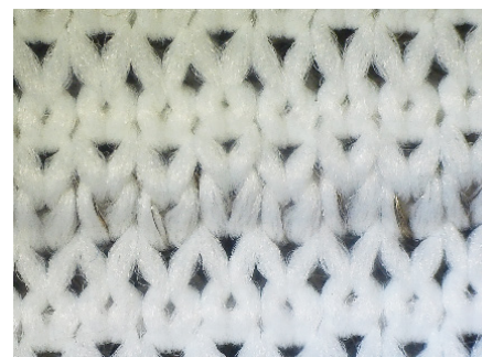
FIGURE 49: PLATING BACK SIDE: ALMOST PERFECT
