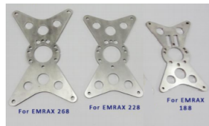
Figure 6.2: Brackets to mount the engines
