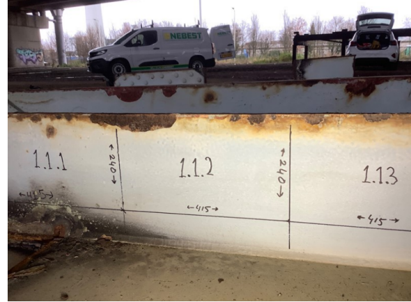
(b) Marked locations for specimen extraction.
