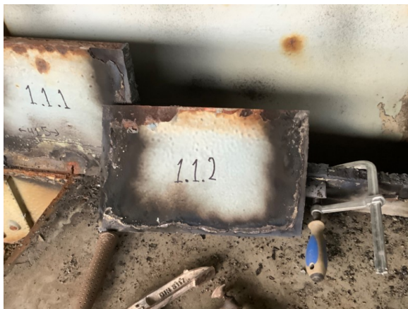
(c) Steel section after extraction from the original member.
