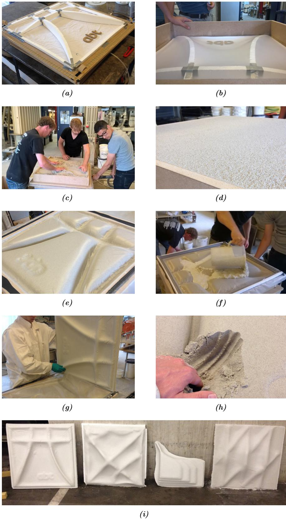
Figure 5.4: 'Vacuumatic Formwork' workshop at the ISOFF-IASS 2015 symposium
