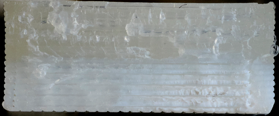
Figure 58: Crosssection break rPLA specimen 2
