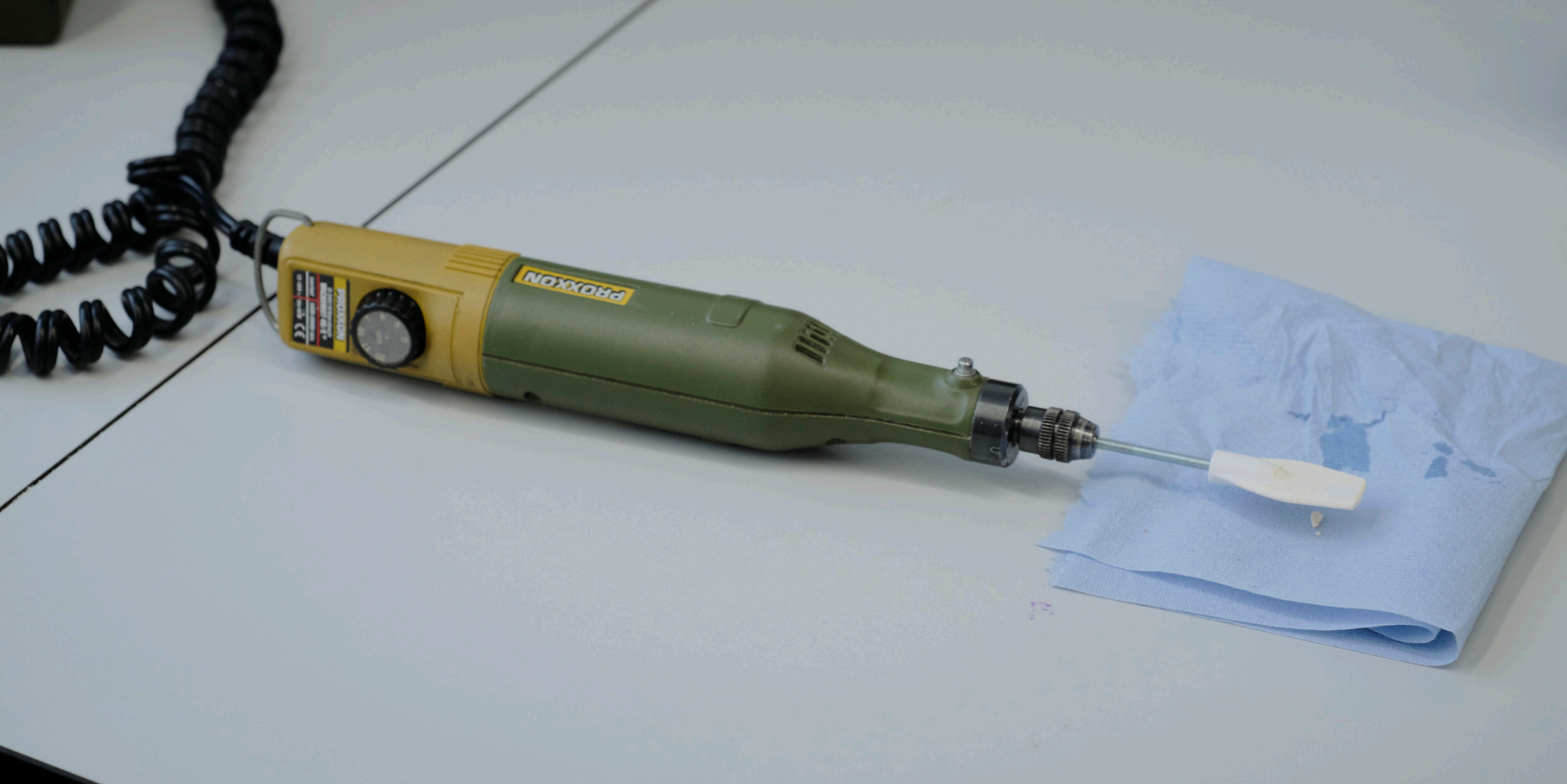
Figure : A Proxxon Micromot 40/e with custom mixing bit was used for mixing materials
