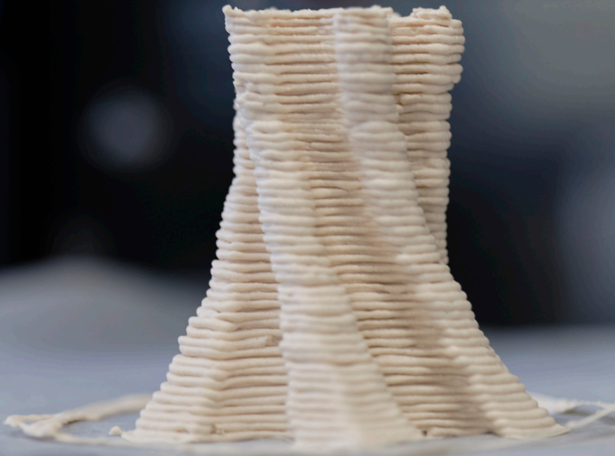
Figure 2: Vase print using final material mix recipe
