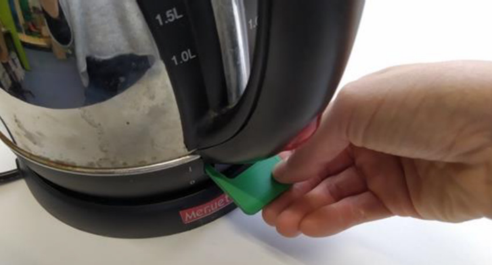
Figure 5: AM can be used for repairing products (Flipsen and Faludi, n.d.)
