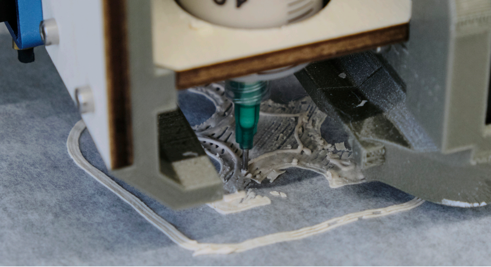
Figure 40: High Travel Speed Damaging Prints
