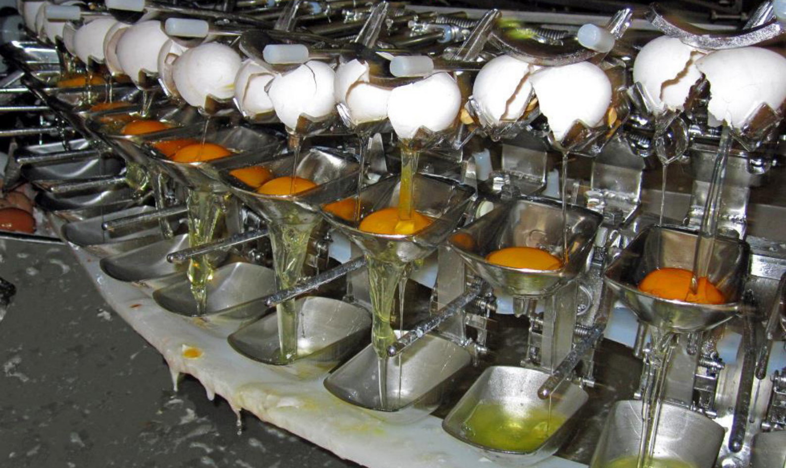
Figure 26: Egg separation at breaker plant (Aaron Equipment Company, 2022)
