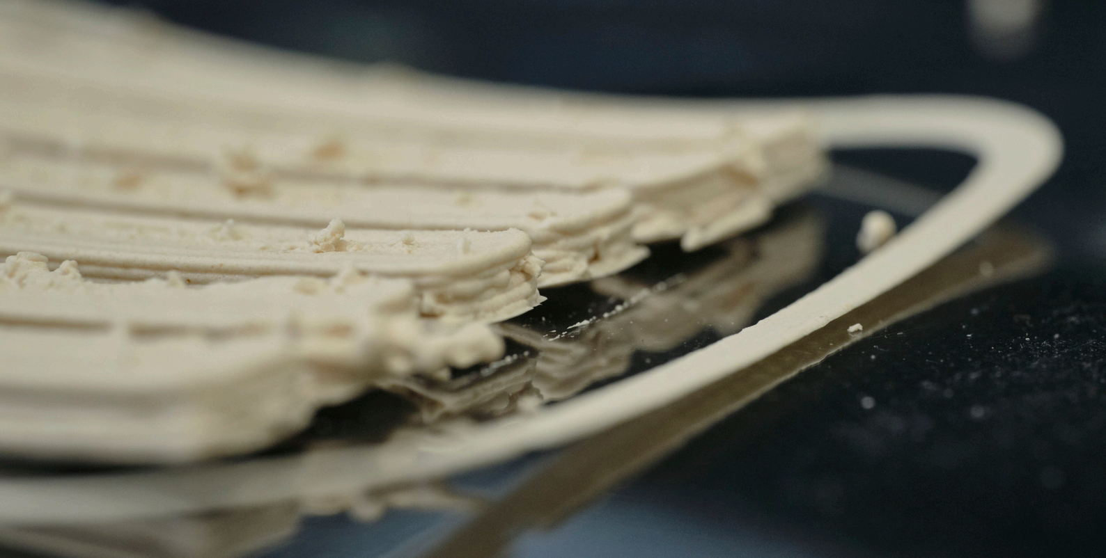
Figure 51: Warping of bending specimens suggested
