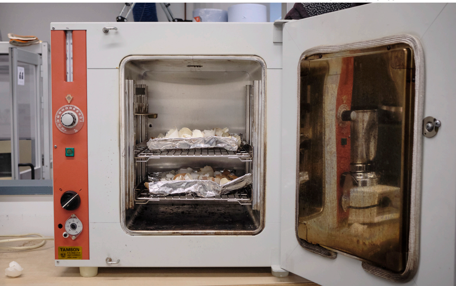
Figure 20 Drying eggshells in oven
