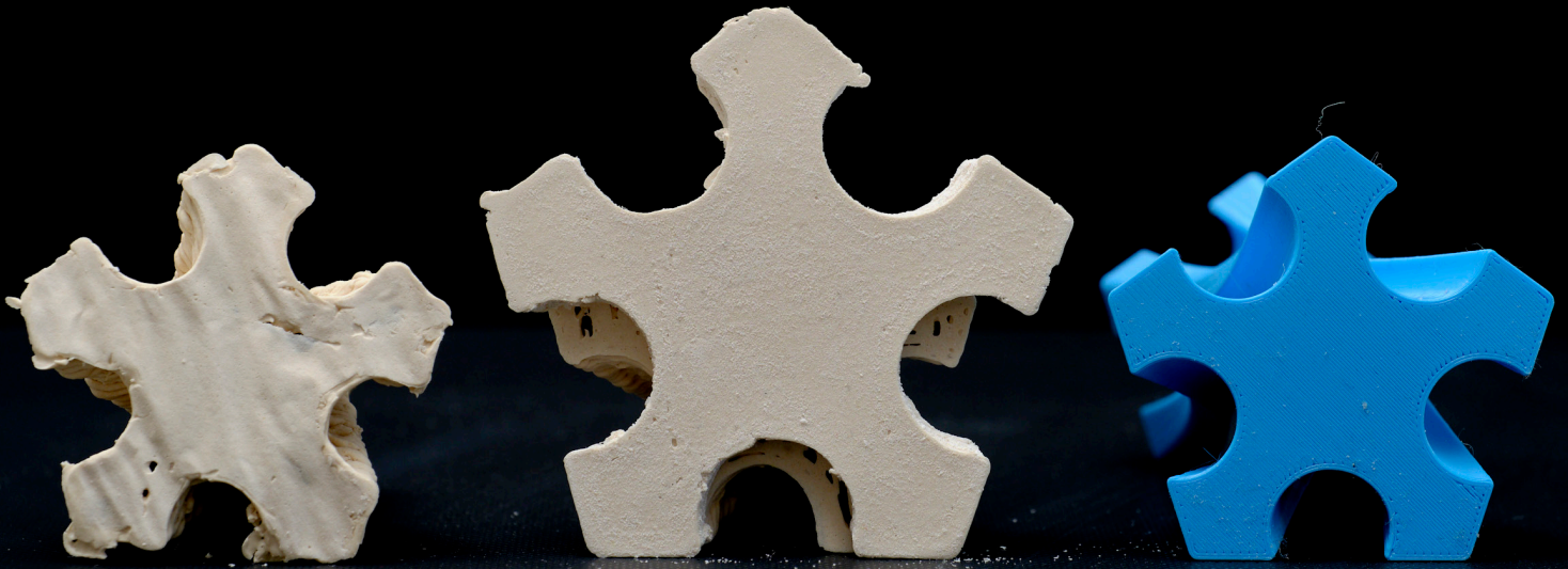
Figure 14: Bottoms of prints. Material mix on baking paper (left), material mix on plastic sheet (middle) rPETG on metal-coated printbed (right)
