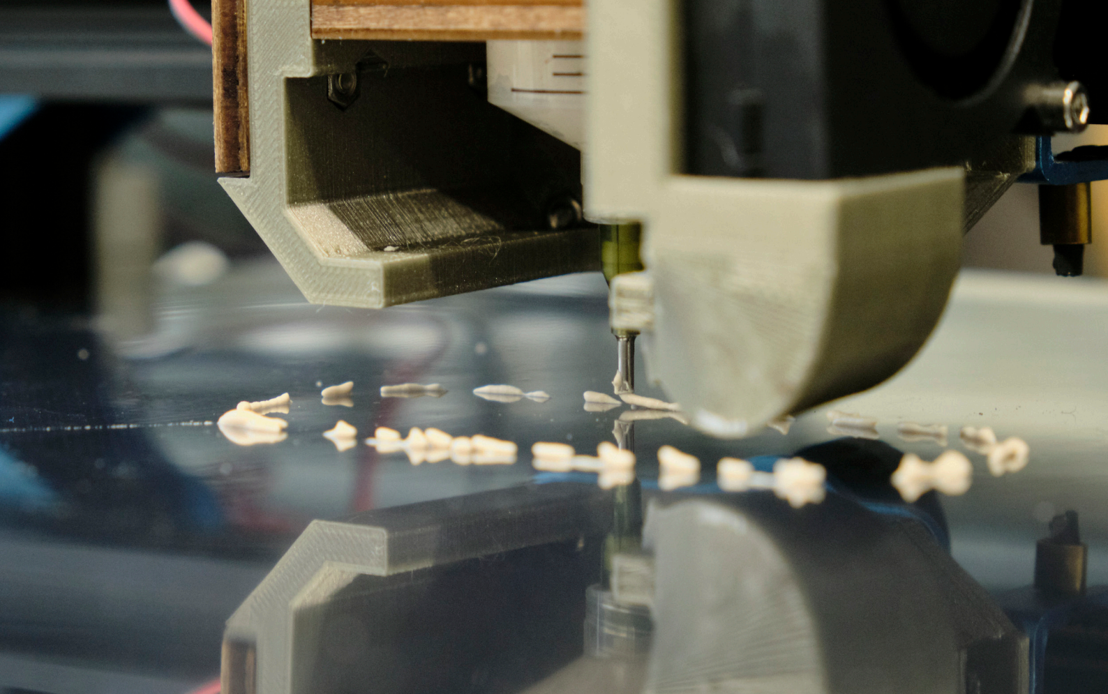
Figure 47: Extrusion may not start out well
