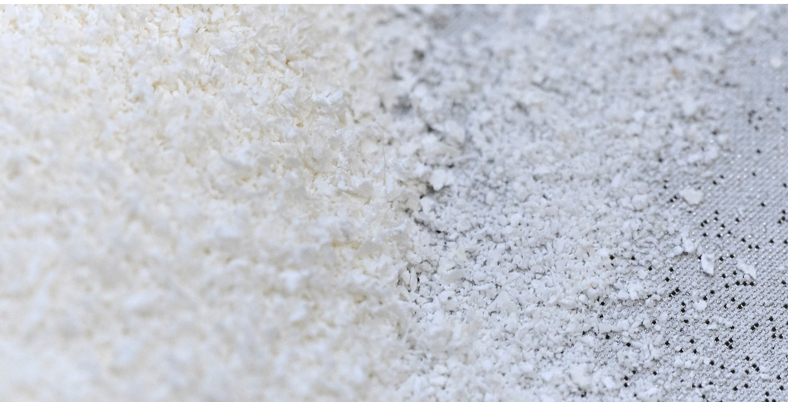
Figure 22: Sieving eggshell flour to get more homogeneous particle sizes
