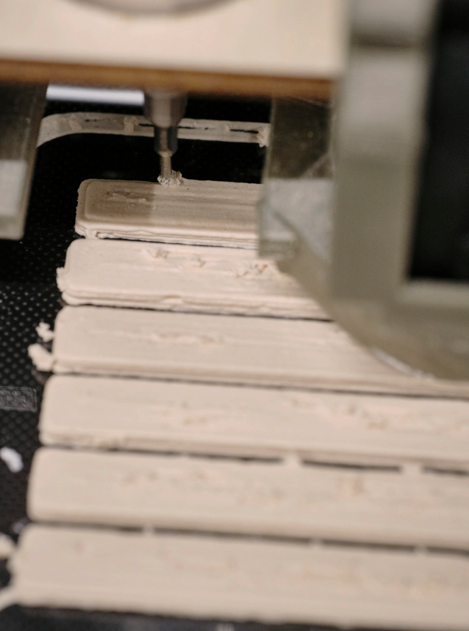
Figure 48: Printing of bending specimens
