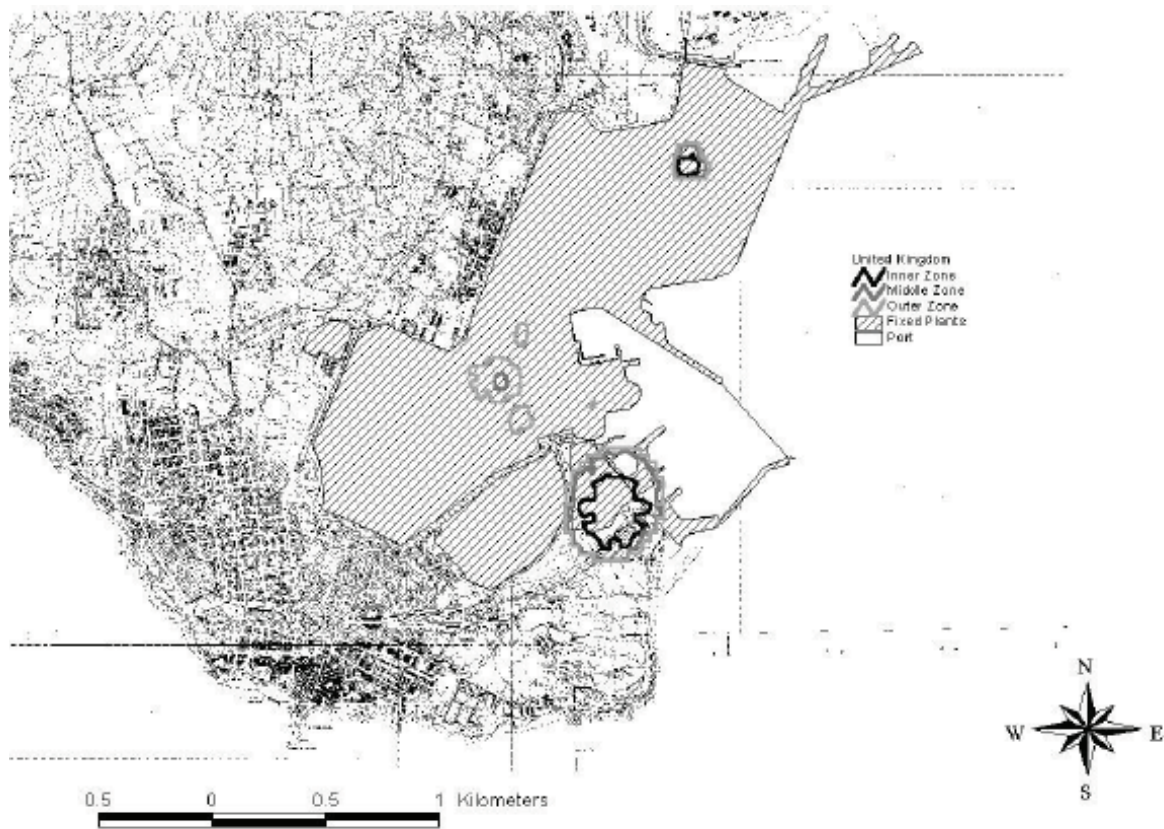
Fig 27 – Application of the British LUP criteria after the four proposed hazard reduction actions (from Cozzani et al 2006)
