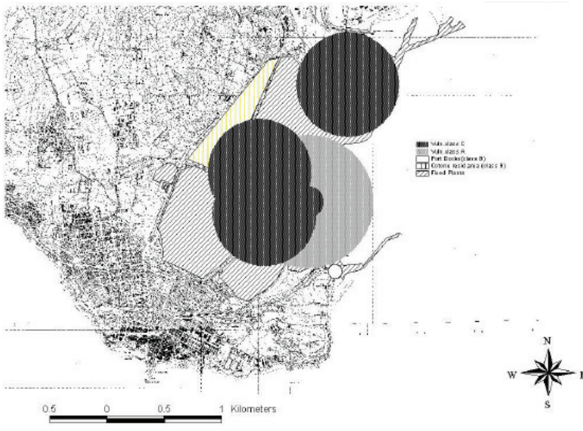
Fig 28 – Application of the Italian LUP criteria after the proposed four hazard reduction actions (from Cozzani et al 2006)
