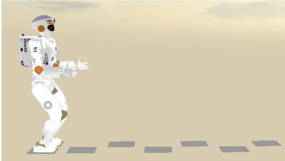
Figure 6-1: Test setup for push recovery during walking in simulation. The limited foothold options show that footstep adjustment is not available as a balance strategy.
