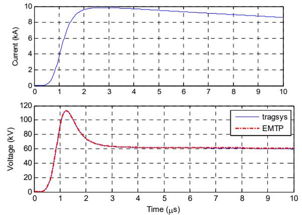
Fig. 7. Current impulse 1.2/50  $\mu$ s and corresponding ground potential rise at the arrester grounding point.
