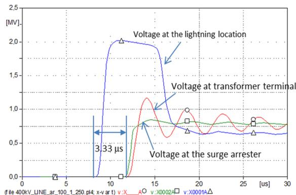
Fig. 18. Overvoltages on the lightning arrester and transformer terminals when the lightning with 10 kA, 1.2/50  $\mu$ s occurs on 1 km distance from the transformer.
