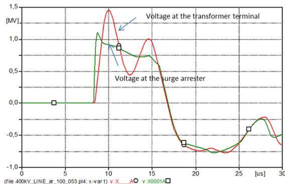
Fig. 17. Voltage response when the system is exposed to LI, 0.5/3 us, 30 kA, 100  $\Omega$ m.
