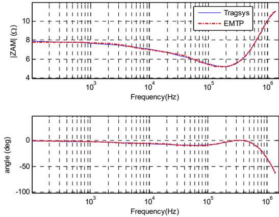
Fig. 10. Amplitude and phase characteristic of the mutual impedance  $Z_{AM}$  between the arrester earthing point AA and the middle point MM of the grounding system for a specific soil resistivity of 1000  $\Omega\text{m}$ .
