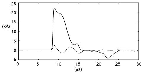
Fig. 20. Current injected into the grounding system for the case of lightning current of 30 kA 0.5/3  $\mu$ s and soil resistivity 100  $\Omega$ m. Full line – at arrester grounding point. Broken line – at transformer.
