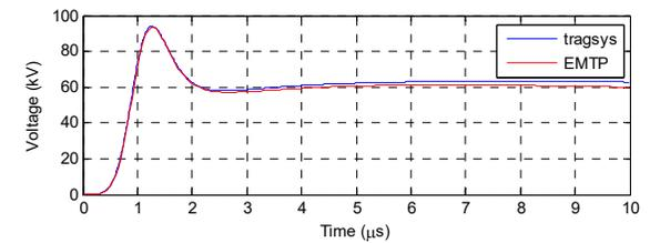
Fig. 9. Ground potential rise in the middle of the grounding system.
