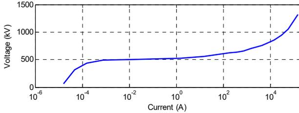
Fig. 14. Lightning arrester characteristic.
