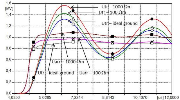
Fig. 16. Comparison between transformer voltages for different specific soil resistivity and ideal grounding for a discharge current 25 kA, 1.2/50 μs.
