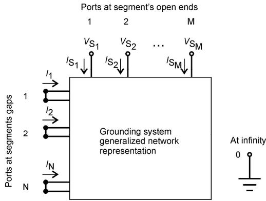
Fig. 4. Generalized network representation of the grounding system
