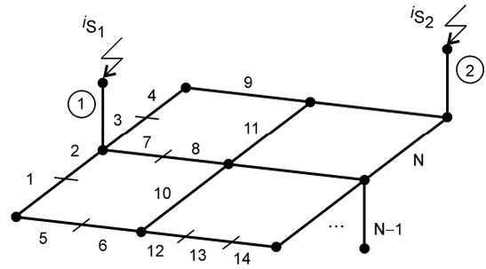
Fig. 1. Grounding system model divided in fictitious segments.
