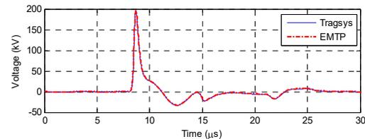
Fig. 19. Voltage at the arrester grounding point AA computed by Tragsys and EMTP for the case 30 kA 0.5/3  $\mu$ s and soil resistivity 100  $\Omega$ m.
