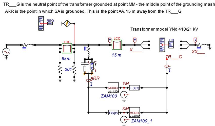
Fig. 13. Representation of the studied system modelling in ATPDraw.
