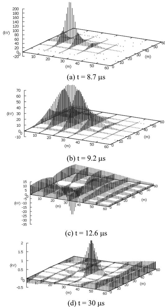
Fig. 21. Snapshots of computer animation of the potential distribution at grounding conductors computed by Tragsys for the case of lightning current of 30 kA 0.5/3  $\mu$ s and soil resistivity 100  $\Omega$ m.
