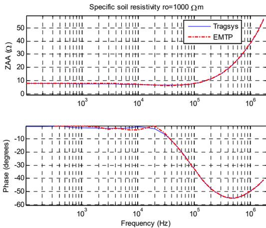
Fig. 6. Amplitude and phase characteristic of the impedance  $Z_{AA}$  at the arrester grounding point of the grounding system, for the soil resistivity of 1000  $\Omega$ m.
