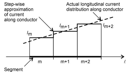
Figure 2. Actual longitudinal current distribution along conductor axis and its stepwise approximation.
