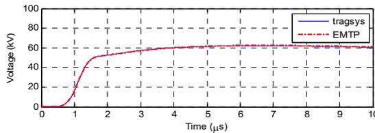
Fig. 11. Ground potential rise at the arrester grounding point when the lightning stroke is injected in the middle point the grounding system.
