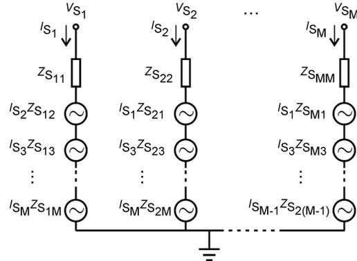
Fig. 5. A grounding system equivalent circuit seen from the above ground power system.
