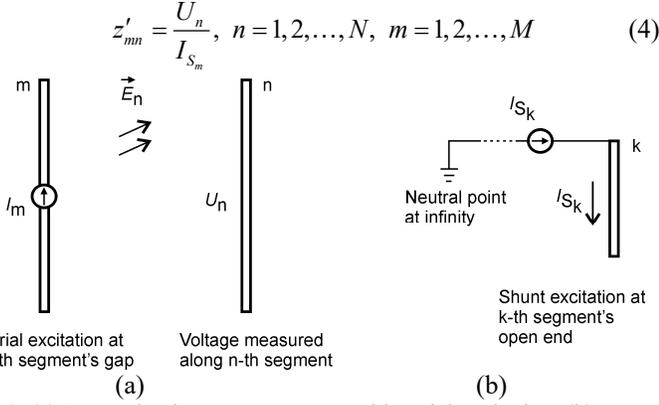
Fig. 3. (a) Interaction between segments with serial excitation; (b) Segment with shunt excitation.
