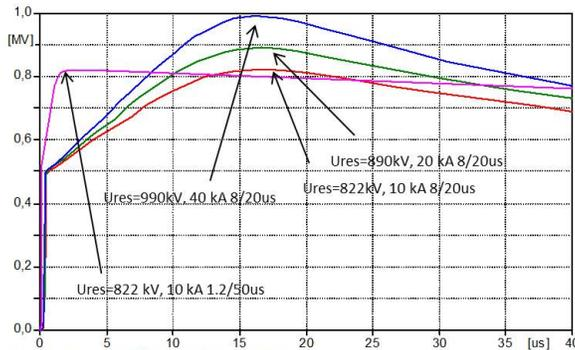
Fig. 15. Results of the residual voltages for different wave shapes.
