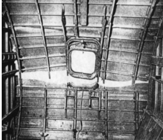
Figure I.1: Fatigue failure at the forward escape window of the De Havilland Comet [5]
