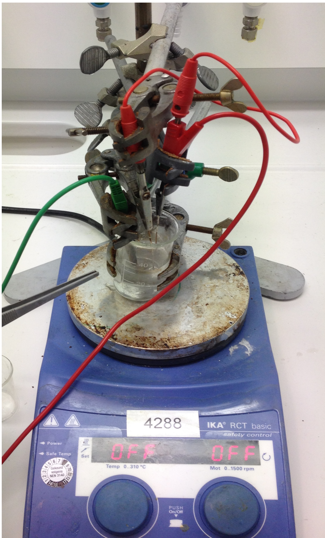
Figure III.1: EP setup, with base heating plate, counter anodes, electrical wires and beaker
