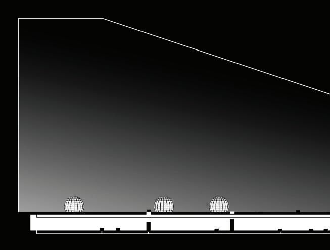
Section of the hangar showing the contrast between the livable pleasant area and the area where harsh wheather is in control. The Globe and the area under the floor with floor heating are kept at pleasant temperatures. Human beings stay close to the floor, up in the air it is too hot or too cold to live. This climate concept creates an energy efficient hangar.
