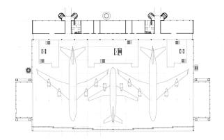
The maintenance hangar on the southern side of the airport cannot be missed. With its hangar space 150 m long, 81 m deep and a clear working height of 26 m, two Jumbo Jets and an Airbus can be dealt with simultaneously.
