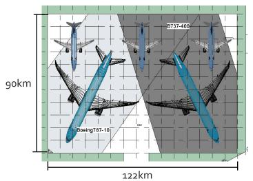
The boundaries for the **footprint** are **90x122 km.** This is based on maintenance on **two Boeing 787-10 and three B737-400 airplanes.** Also other models can be placed in the hangar. All 737 models and th A350 are also possible in this configuration. Larger airplanes are possible but 737's no not fit next to these planes.
