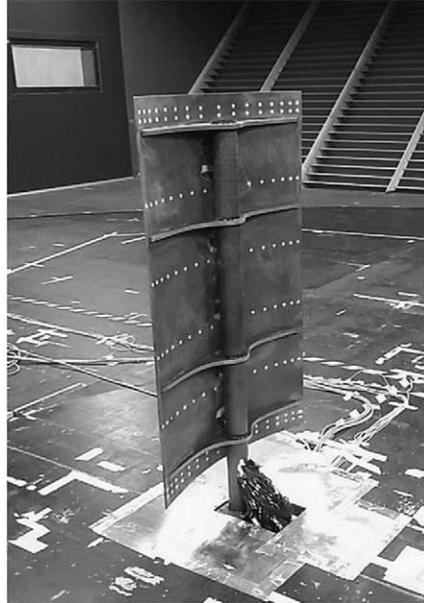
Fig. 1. Sail model used during the experiments.
