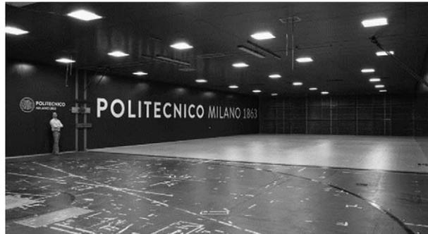
Fig. 4. Wind tunnel boundary layer test section.
