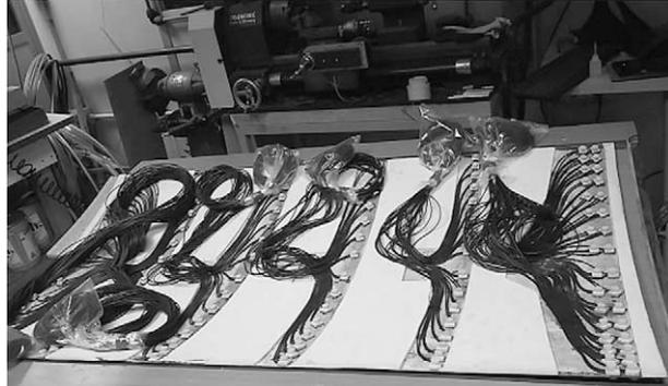
Fig. 2. Assembly of the pressure taps in the sail.
