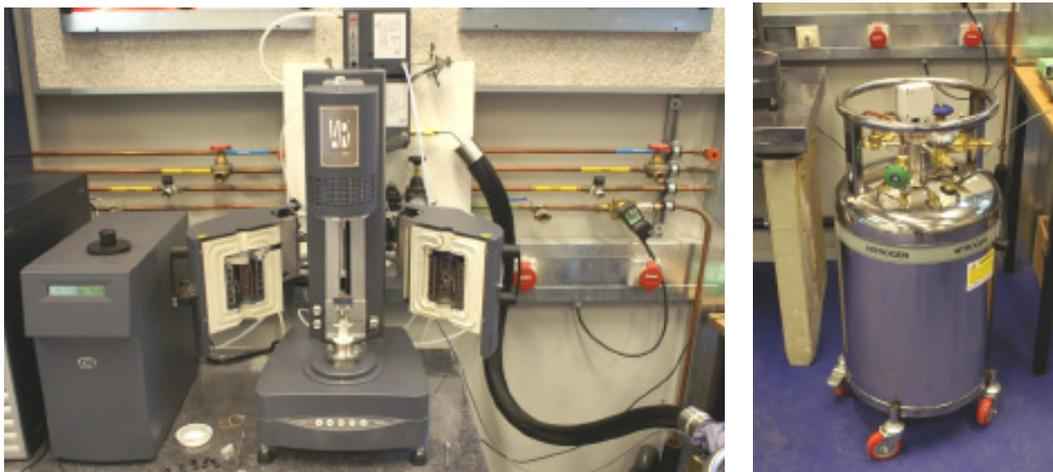
Figure 4-1 DSR environmental test chamber(left); Liquid Nitrogen vessel(right)
