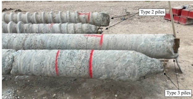
Figure 5. Base of four extracted piles, all installed at the site
