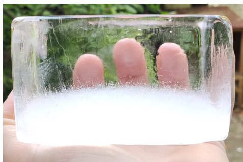
(a) Ice sample created with directional freeze technique; clear ice.
