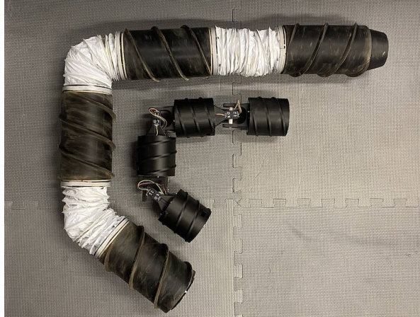
Figure 2.8: ARCSnake together with smaller 'Voodoo Doll', used to control ARCSnake. Image from [65]
