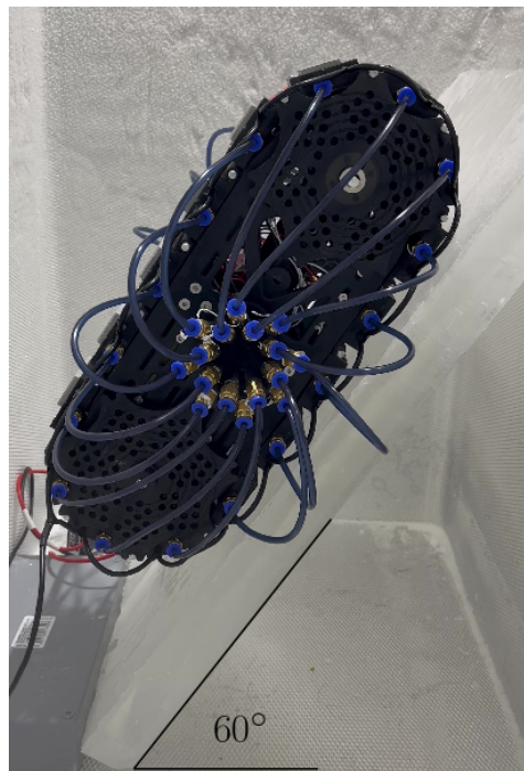
Figure 6.16: Robot climbing a sheet of ice with 60^{\circ} incline.
