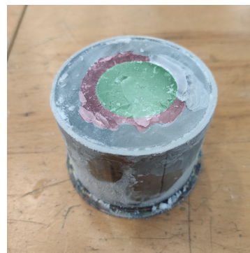
(b) Ice sample 9 after test, failed at F_{\max} = 301 N.
