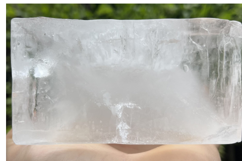
(b) Ice sample created without directional freezing; regular ice.
