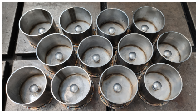
(b) All sample containers with the anchor modification.
