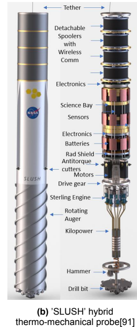
Figure 2.10: Two thermo-mechanical ice probes.
