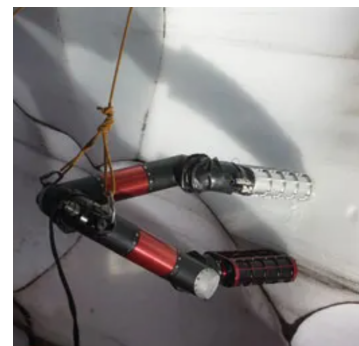
Figure 2.11: IceWorm robot climbing on ice. Image from[13]
