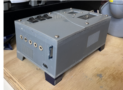
Figure 3.6: Temperature data logger. Part of the thermo-electric cooling setup shown in figure 3.5b.
