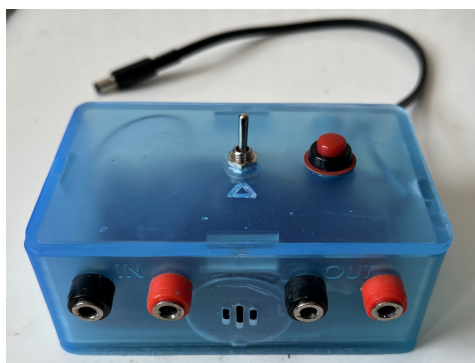
Figure 3.4: H-bridge peltier controller box.
