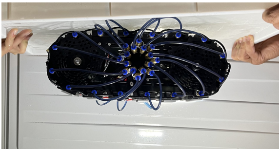
Fig. 14: Robot inverted and anchored to the block of ice.
