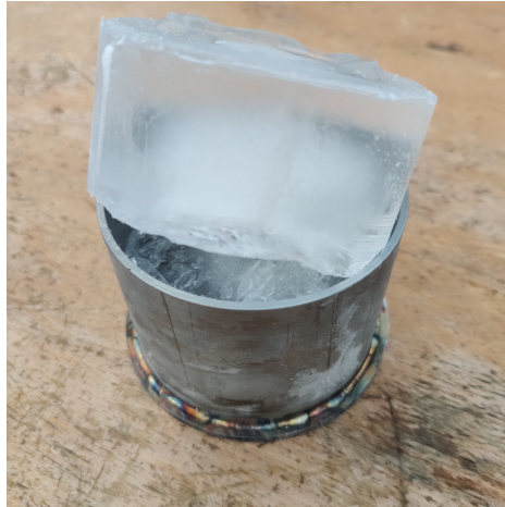
Figure A.19: Cohesive failure of ice sample at bubble interface.
