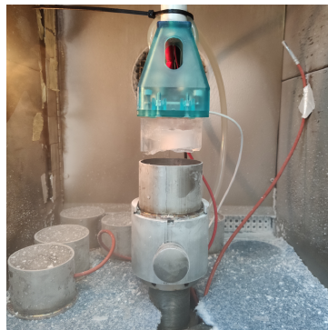
(a) Ice sample attached to the adhesion effector; separated from the container with F_{\max} = 1250 N.
