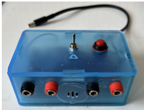
Figure A.12: H-bridge peltier controller box.
