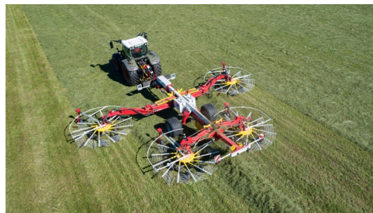
(b) Agricultural hay rake in operation. Image from:[64]
