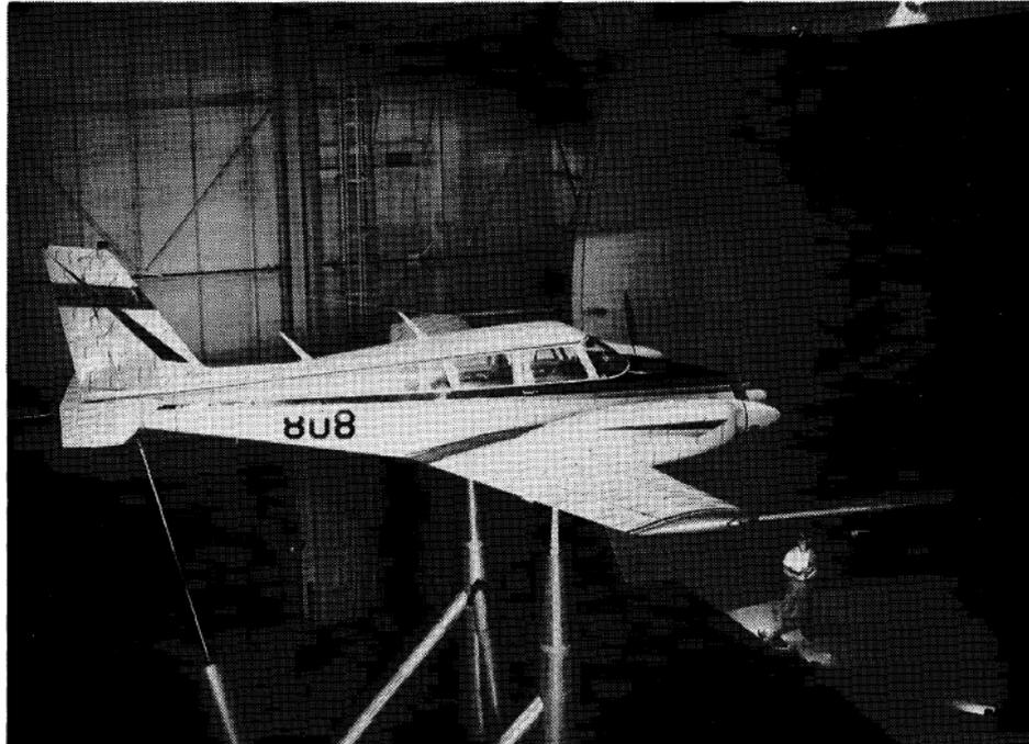
Figure 4.4: Picture of a Piper PA-30 Twin Comanche in a wind tunnel test[50]
