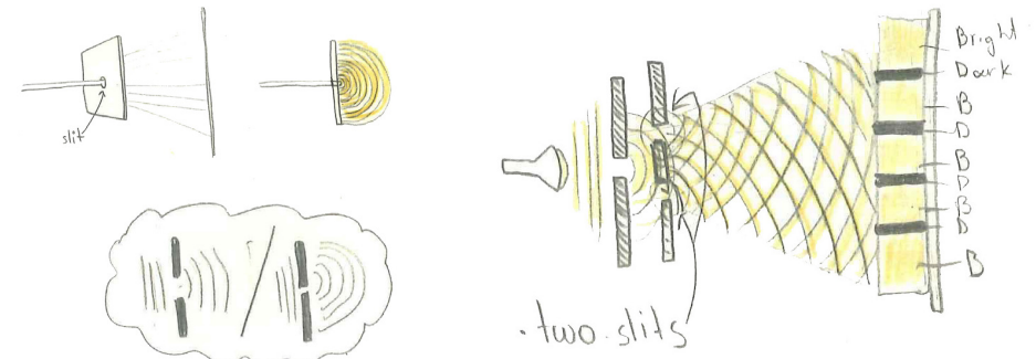
03.b.i. The phenomenon of diffraction of light waves sketch by the author
