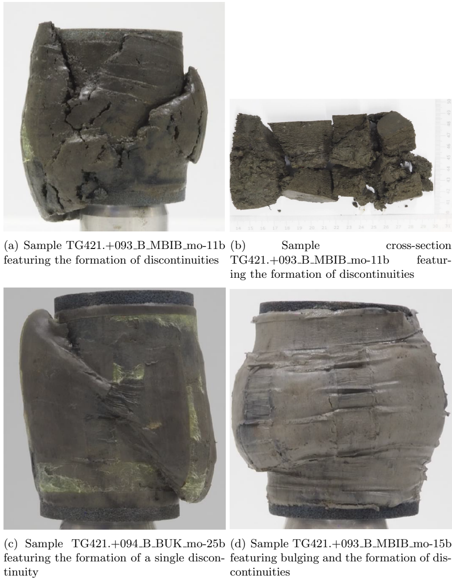
Figure 2.2.3: Typical deformation mechanisms of Gorinchem Clay tested in undrained triaxial from the dry side
