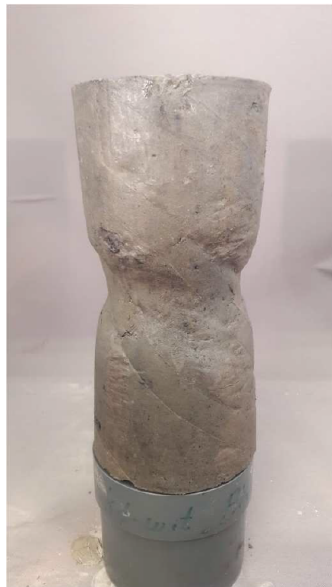
Figure 2.2.5: Typical deformation mechanisms of Gorinchem Clay tested in Undrained Triaxial Extension from the wet side
