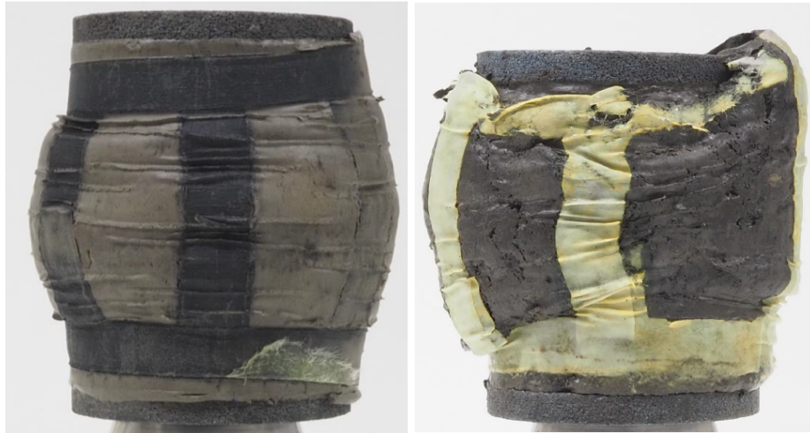
(a) Sample TG421.+094.B.BUT_mo-19b featuring sample bulging (b) Sample TG421.+094.B.BITA_mo-16a featuring sample bulging and formation of discontinuities
