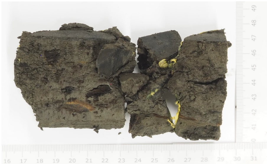
(c) Sample cross-section TG421.+094.B.BITA_mo-16a featuring sample bulging and formation of discontinuities
