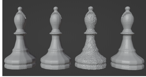
Figure 3: The regularized bishop mesh (left). The regularized bishop mesh with an embedded watermark (left-middle). The regularized bishop mesh with an embedded watermark that has been randomly attacked with a vertex displacement distance of 0.05 (right-middle). The watermarked and attacked mesh after it has been regularized again (right).
