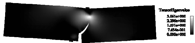
Figure 13. Four-point shear test: maximum principle stress map in the deformed mesh (magnified 200\times ) when CMSD is 0.08 mm for GFEM.
