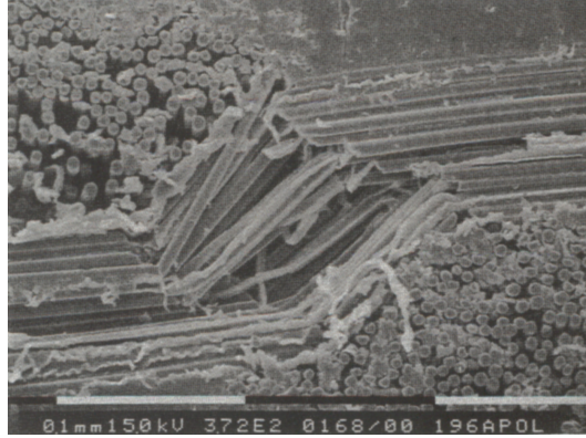
Figure 4.9: SEM-capture of fiber buckling due to compressive loading, adapted from [41]
