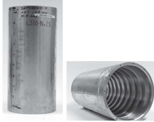
Figure 5.1: Typical internally stiffened cylinder of MacKay's test series [50]
