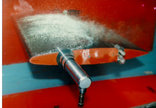
Figure 3.1: Photo of a lifting surface that exhibits a fairly clean "sheet" cavity; near the end of the cavity bubble cavitation occurs. Photograph courtesy of S.A Kinnas, MIT's Variable Pressure Water Tunnel (1996).
