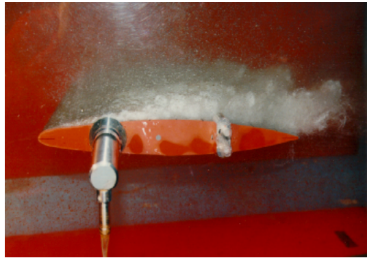
Figure 3.3: Photograph of a hydrofoil exhibiting cloud cavitation. Photograph courtesy of S.A Kinnas, MIT's Variable Pressure Water Tunnel (1996).
