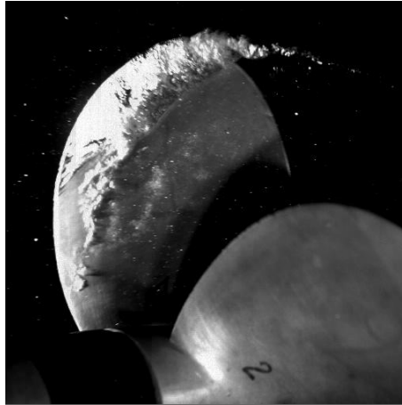
Figure 3.38: Tunnel flow visualization of the INSEAN E779A propeller model during experimental investigation.
