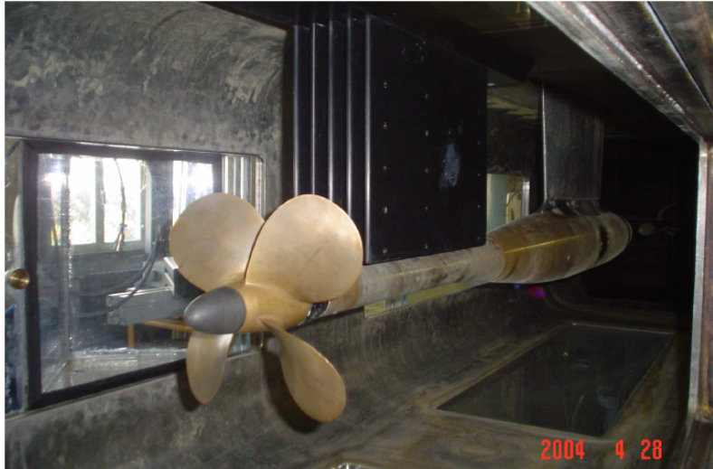
Figure 3.39: INSEAN E779A propeller model inside the cavitation tunnel.
