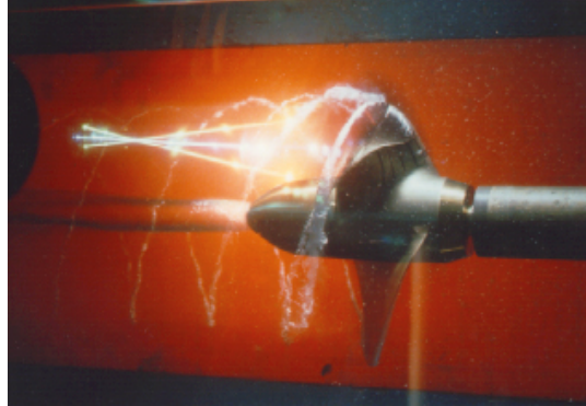
Figure 3.4: Photograph of a cavitating propeller in presence of tip-vortex cavities and hub-vortex originating from the tip and the hub of the propulsor. Photograph courtesy of S.A Kinnas, MIT's Variable Pressure Water Tunnel (1996).
