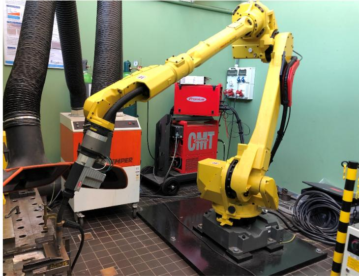
Figure 3.2: Robotic welding system
