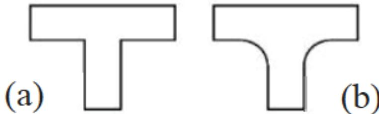
Figure 2.10: Internal corners of T crossing structures; (a) sharp (b) with fillet [12]
