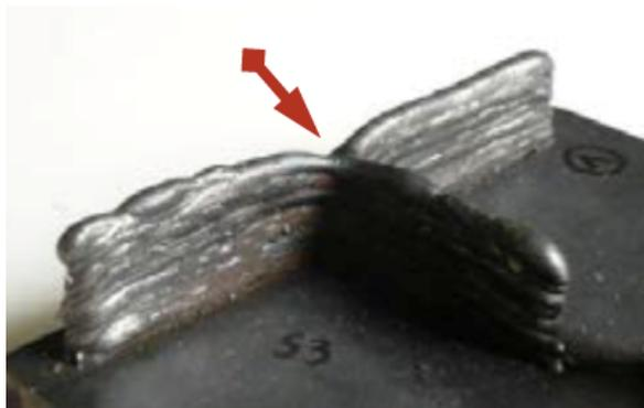
Figure 2.14: T-crossing structure built by strategy 3 (S3); the red arrow points at the deposition failure in the central zone [12]
