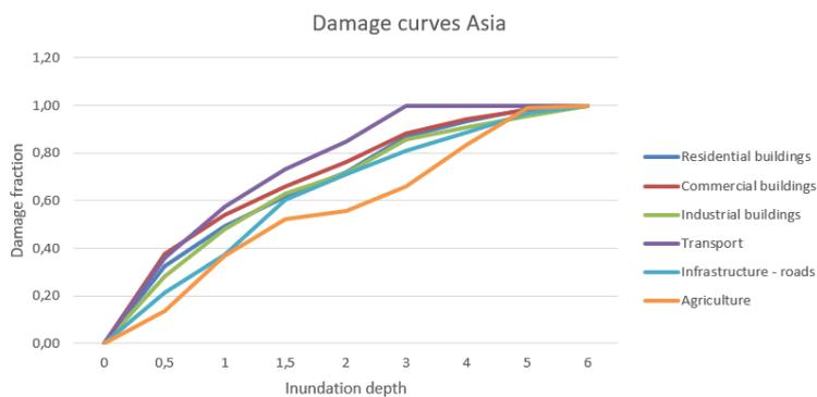
Figure F.1: Damage functions for Asia (Huizinga et al., 2017)
