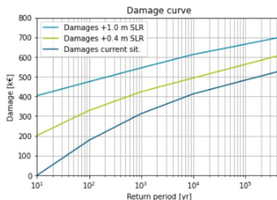
**Figure 4.4:** The damages for different water levels
