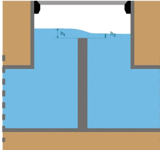
Figure A.1:  $h_1$  and  $h_2$  visualised (RioNed, 2019)
