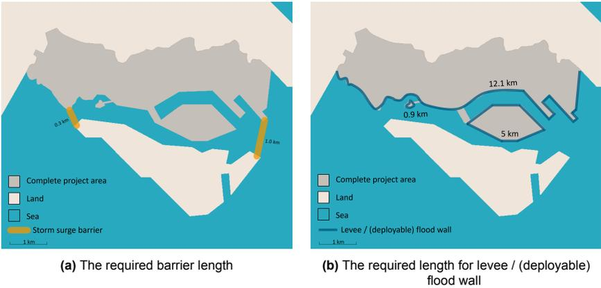
Figure 5.19: The required dimension of the measures
