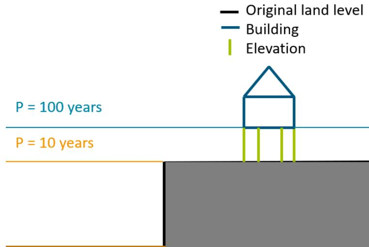
**Figure 3.4:** An illustration of the safety level of Dryproofing / Elevation
