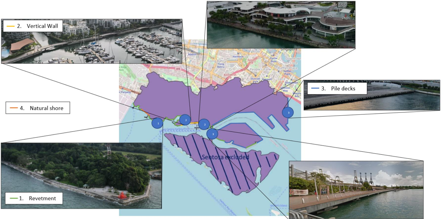
Figure 5.5: The current coastal protection with self-taken pictures supplemented with pictures of Google Maps
