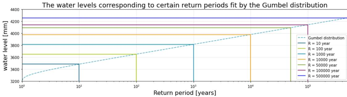
Figure 5.9: The Gumbel distribution fitted through the adjusted water levels
