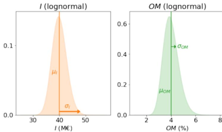
**Figure 2.3:** Example distributions of the considered stochastic variables  $I$  and  $OM$  with the adjustable parameters  $\mu_I$ ,  $\sigma_I$ ,  $\mu_{OM}$  and  $\sigma_{OM}$  (Dam, 2021)
