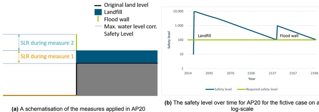
**Figure 4.6:** Schematisation of AP20
