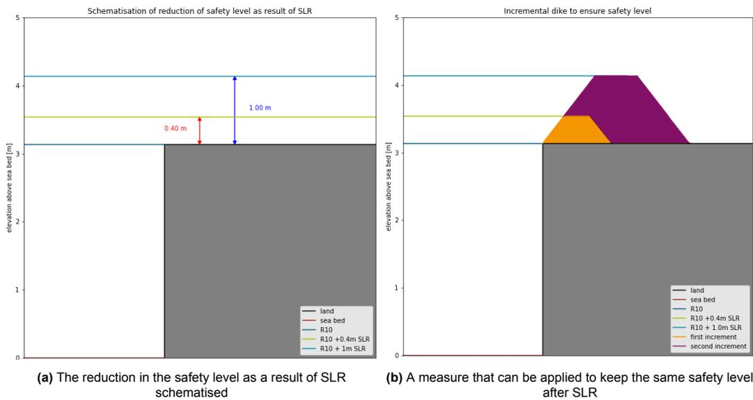
Figure 4.3: The consequence of SLR schematised
