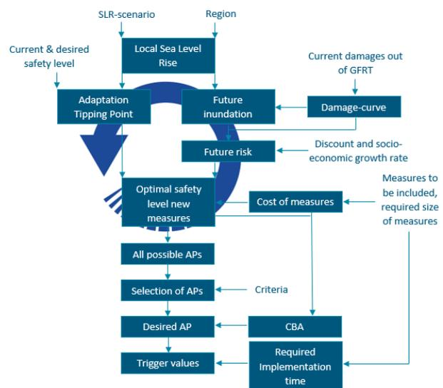
Figure 3.1: The outline of the constructed tool
