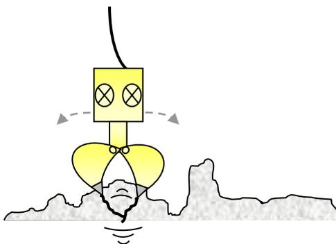
Figure 21: Situation overview of grab excavating rock on seafloor.
