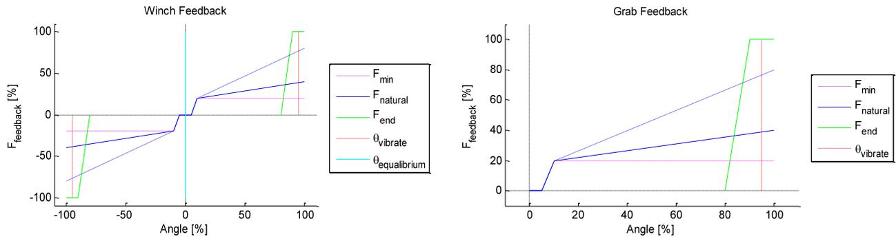
Figure 36: a) Illustration of the force feedback mechanisms of the winch joystick. b) Illustration of the force feedback mechanisms of the grasping joystick.
