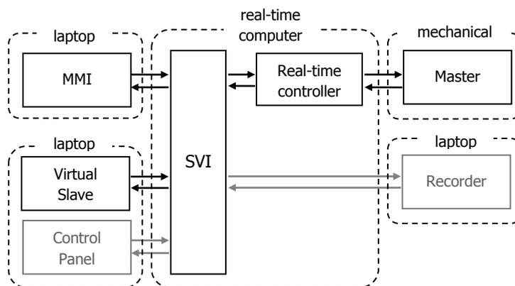
Figure 30: Software structure of the experimental setup
