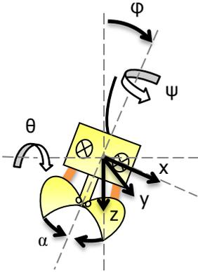
Figure 2: Degrees of freedom of a suspended grab, shown in coordinates of control
