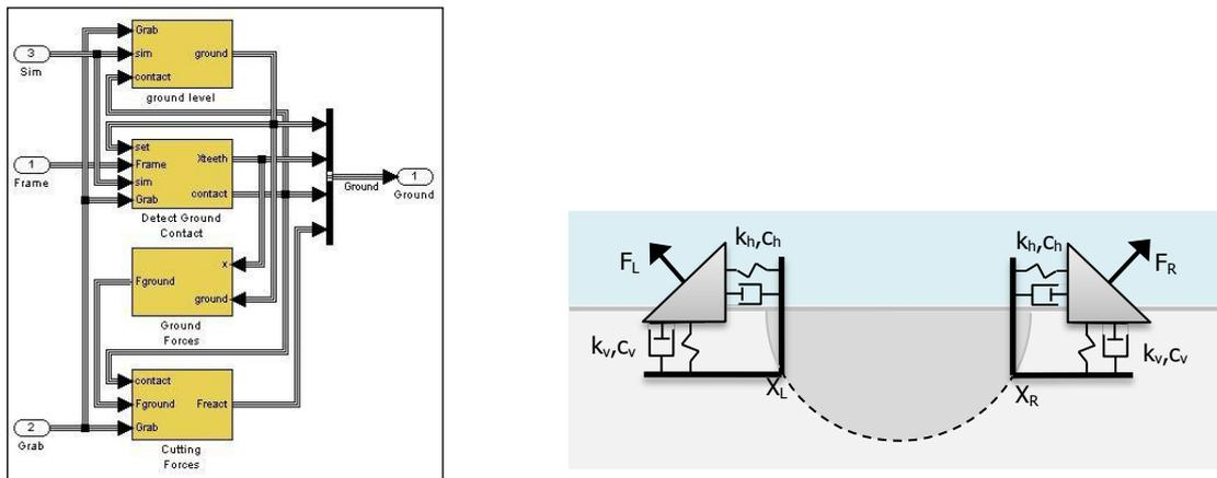
Figure 42: a) A Matlab Simulink representation of ground contact and force calculations. b) Schematic representation of mass-spring system for ground contact forces for changing ground positions.
