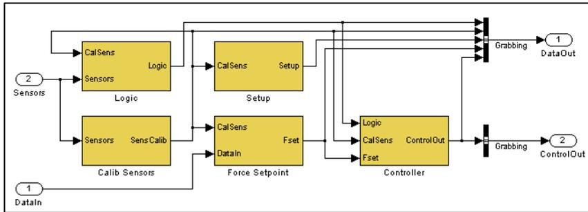
Figure 34: A Matlab Simulink representation of the grabbing control part of the real-time controller
