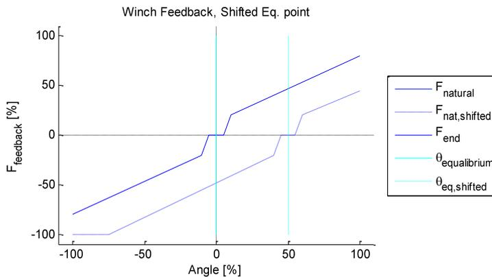
Figure 37: Illustration of the mechanism of shifted equilibrium point of the continuous haptic shared control feedback mechanisms for the winch joystick.
