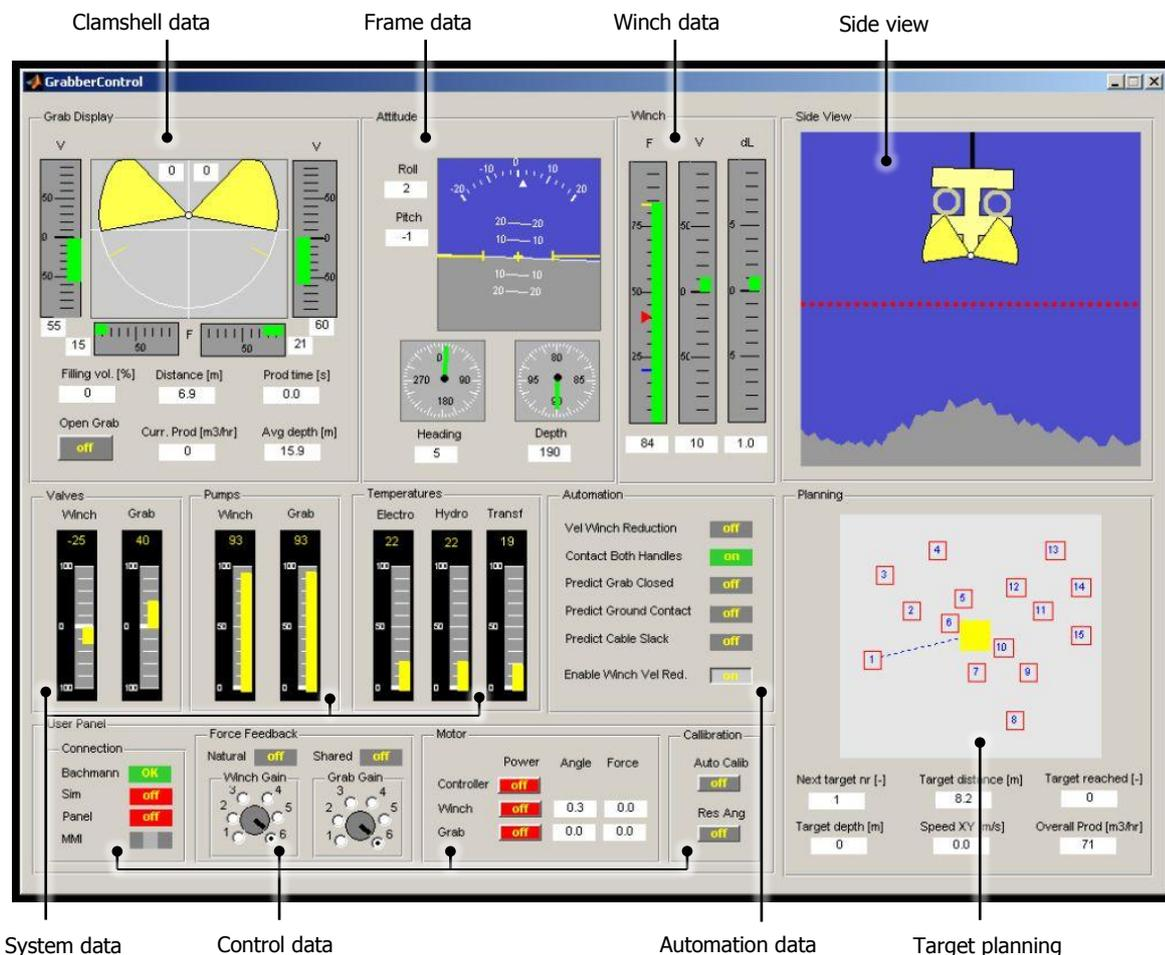
Figure 31: Visual interface for controlling a deep sea mining process
