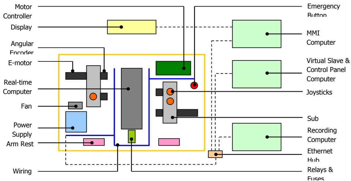
Figure 29: Schematic view of mechanical and electrical components of experimental setup
