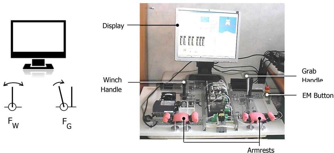
Figure 20: a) Schematic view of experimental setup with a display and two joystick handles. b) Overview of experimental setup with two joysticks and display.
