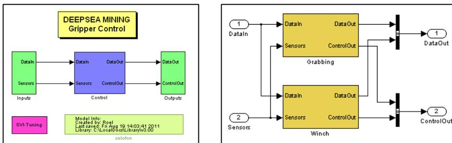
Figure 33: a) Top level of control model as implemented in Matlab Simulink. b) Control of the real-time controller, showing two control parts for the grasping and winch joystick.
