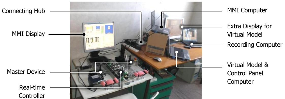
Figure 25: Complete overview of experimental setup with all connected hardware for controlling the setup.
