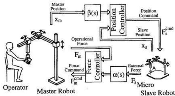
Figure 11: Transparent Feedback Application with impedance shaping scale factors (adapted from Kaneko et al. 1997 [20], pp. 71).
