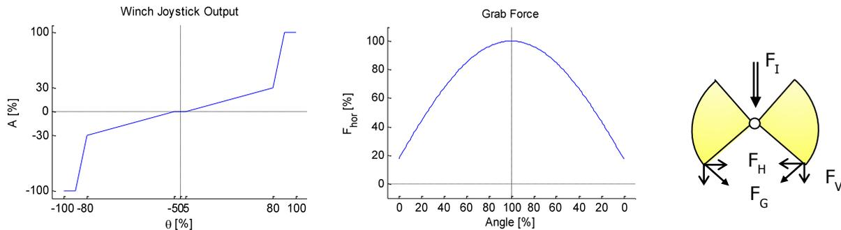
Figure 44: a) Non-linear winch joystick output b) Non-linear grab force c) decomposed grab forces.
