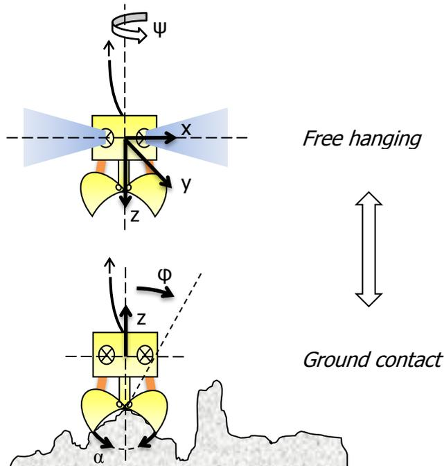
Figure 7: Change of grab movement during contact transition
