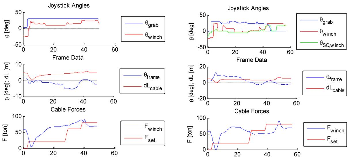
Figure 49: a) Time trace results of performance task 1 for subject nr.6 using direct control (DC) as experimental condition, showing the control action of joystick angles and reaction of the slave robot simulation of relative cable length, heeling angle and cable force with controller setpoint. b) Time trace results of performance task 1 for subject nr.6 with Haptic Shared control feedback (DC-SC) showing identical parameters, including the feedback parameter for the winch joystick.
