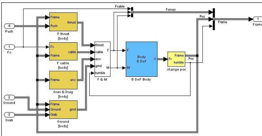
Figure 41: A Matlab Simulink representation of the calculations of the grabs frame dynamic behaviour.
