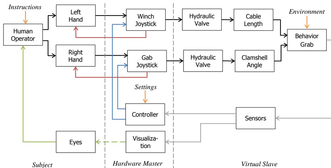
Figure 4: System control overview for tele-operating a remotely controlled grab. Red lines indicate feedback on human hand, blue lines current on electric motors, green lines visual feedback and orange lines system inputs.
