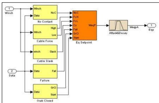
Figure 43: Calculation of equilibrium point for winch shared control
