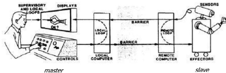
Figure 8: Schematic view of a teleoperation with visual feedback (adapted from Sheridan 1989 [33], pp. 2)
