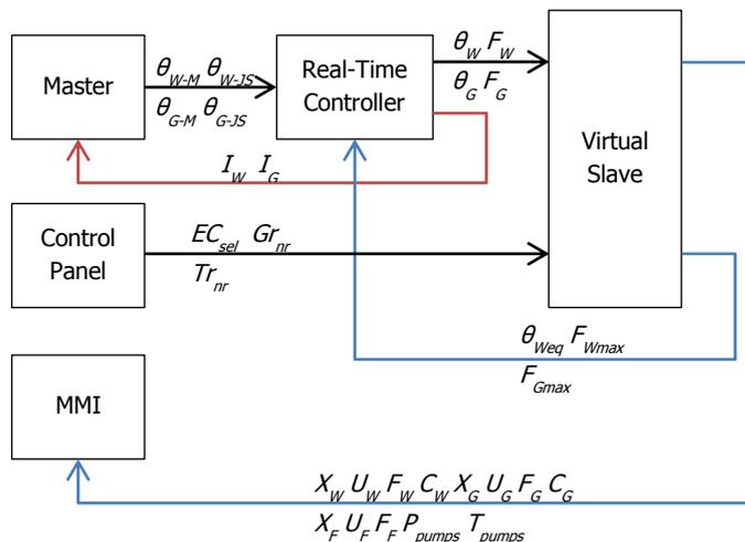
Figure 39: Schematic view of communication of the virtual grab model.
