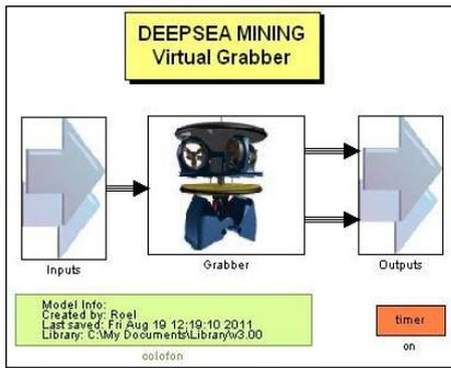
Figure 38: Top level of Matlab Simulink representation of the virtual grab model.
