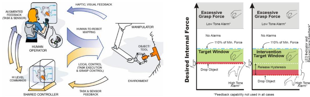
Figure 19: a) Schematic representation of Grasping Objects with Shared Control (adapted from Griffin et al. 2003 [12], pp. 1). b) Methods of feedback to the operator for grasping with shared control (adapted from Griffin et al. 2003 [12], pp. 3).
