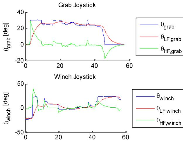
Figure 50: Decomposition of low and high-frequent control movement of joystick angles for subject nr.6 using haptic shared control (DC-SC) condition during performance task 1.
