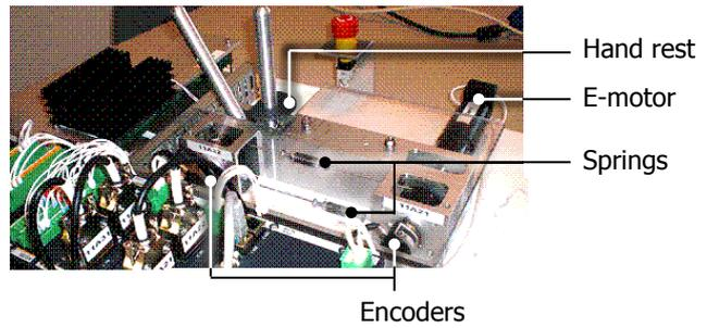
Figure 26: a) Schematic view of mechanical principle for a single joystick. b) View of experimental setup for the grabbing joystick.
