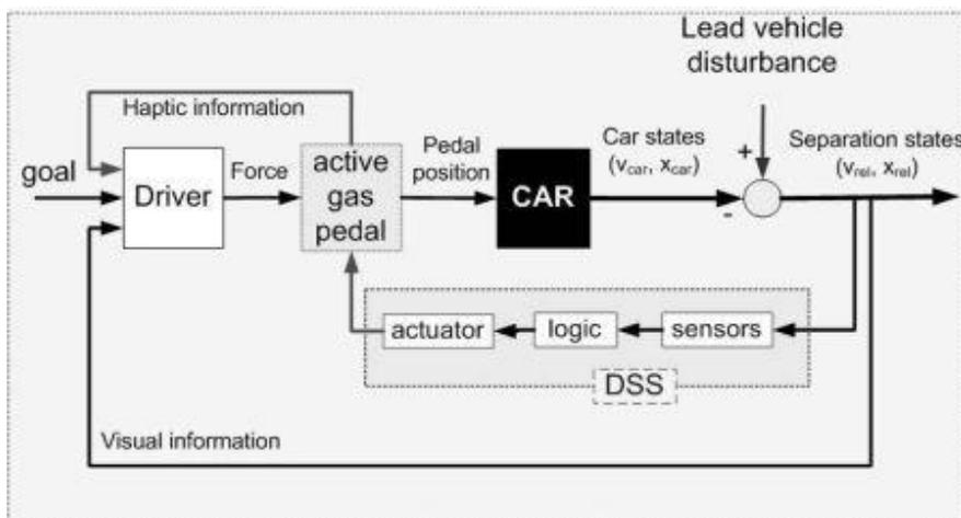
Figure 17: Shared Control Algorithm for car following with guiding haptic force feedback (adapted from Abbink 2006 [1], pp. 7)
