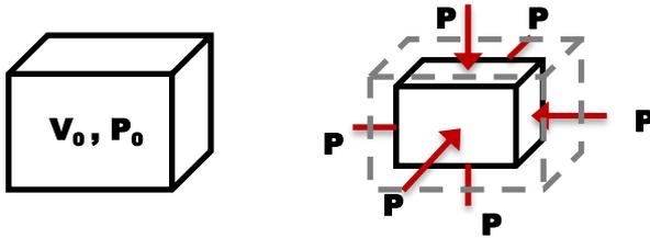
Figure 6: Principle of uniform compressed hydraulic volume.
