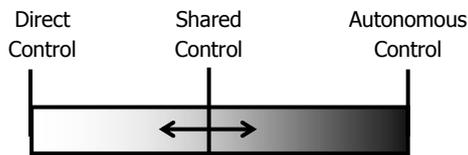
Figure 13: Schematic view of principle of haptic shared control, for continuous shift of authority.
