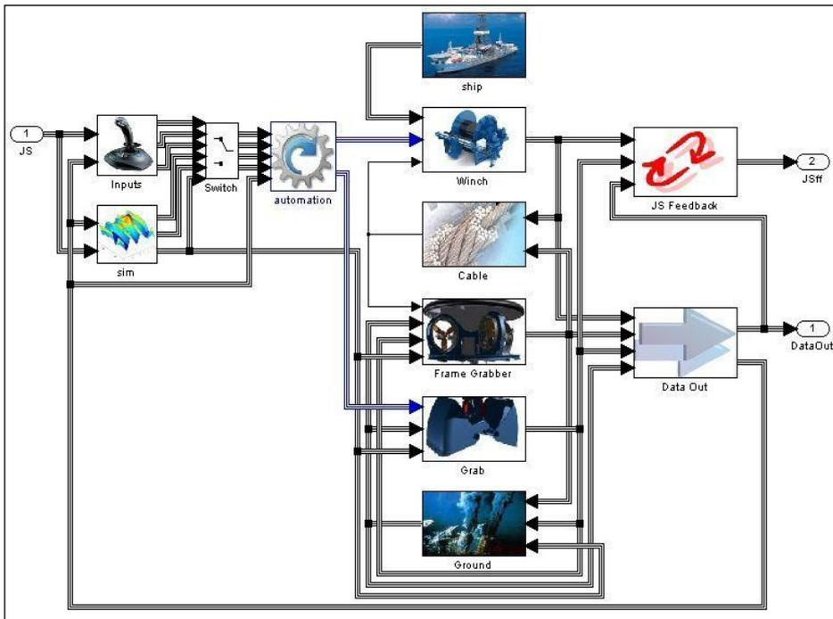
Figure 40: A Matlab Simulink representation of the virtual grab simulation model, subdivided into physical separated parts.
