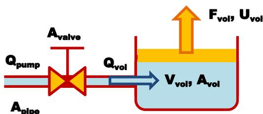
Figure 5: Schematic view of principle of hydraulic volume with controlled inflow
