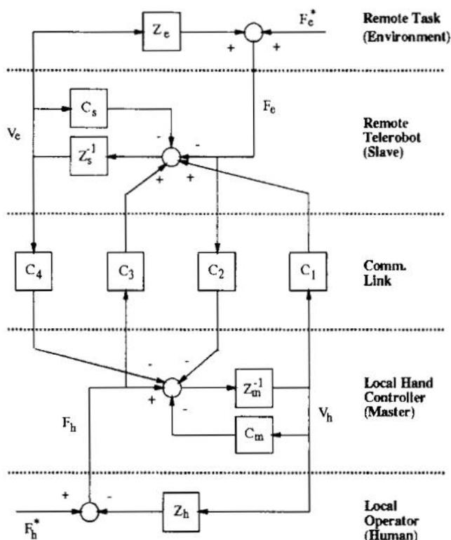
Figure 12: Transparent feedback control algorithm using a four channel structure, depicted with gain  $C_1$ -4 of forces and velocities both ways (adapted from Lawrence 1993 [21], pp. 626).
