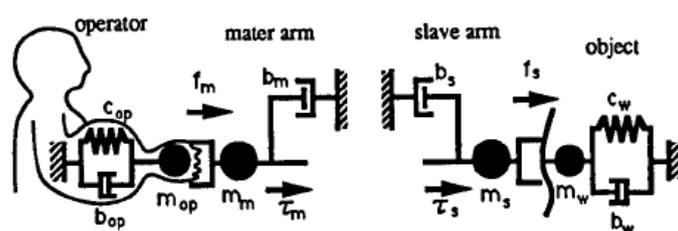
Figure 10: a) Schematic view of dynamics in transparent teleoperation of master and slave arms, operator and object (adapted from Yokokohji 1992 [40], pp. 850).
