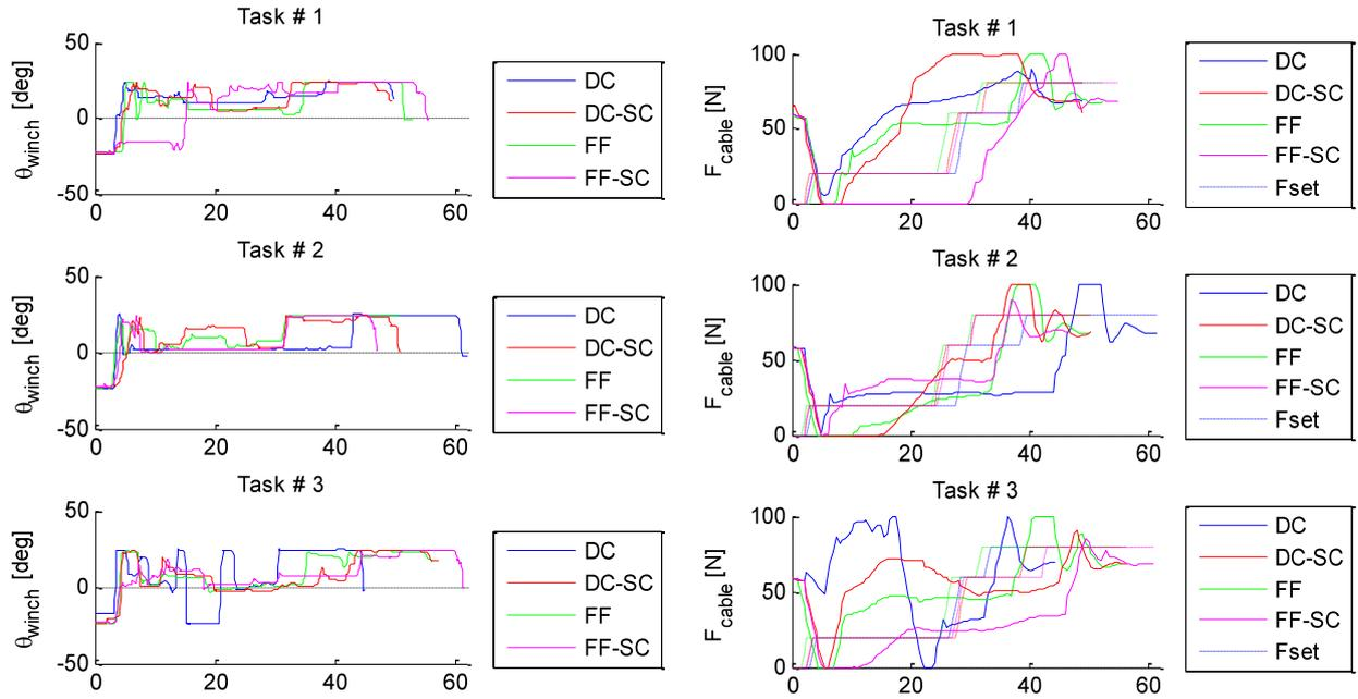
Figure 48: a) Time trace results of winch joystick rotation angles of subject nr.6 during all three performance tasks. b) Time trace results of cable tension force of the virtual slave robot simulation for all three performance tasks.
