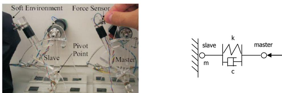
Figure 9: a) A 1 DoF Transparent Feedback Mechanism experiment for contact probing (adapted from Abbot and Okamura 2003 [2], pp. 2). b) Schematic representation of 1 DoF transparent feedback mechanism with artificial mechanical properties; mass  $m$ , stiffness  $k$  and damping  $c$ .
