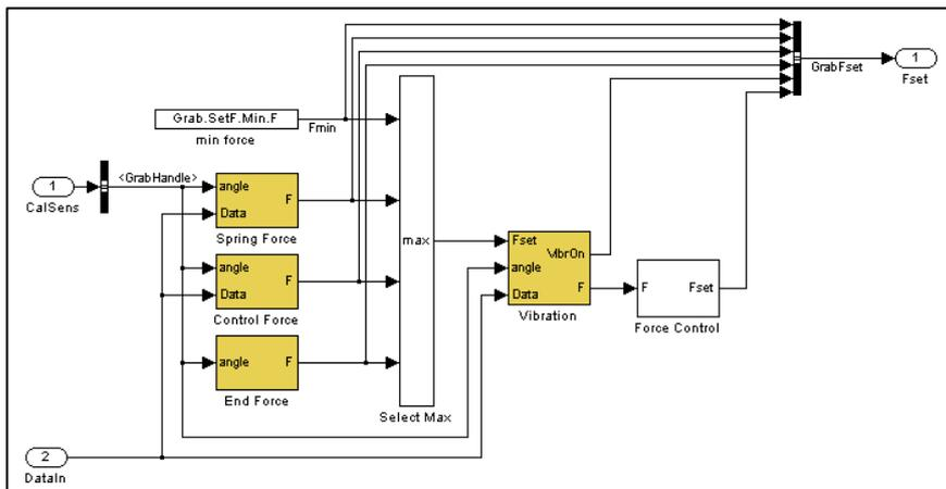
Figure 35: Matlab Simulink representation of force setpoint calculation, depending on different components
