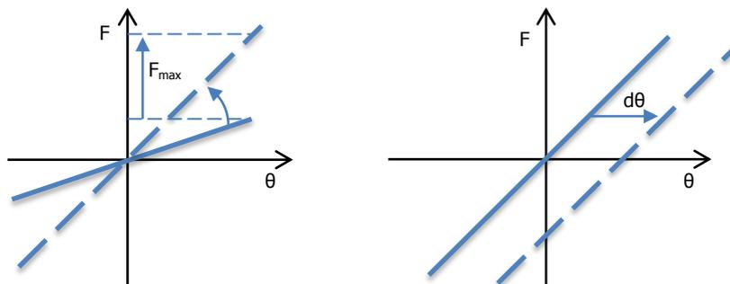
Figure 22: a) Stiffness feedback mechanism for haptic feedback on a joystick for natural force feedback. b) Shift of equilibrium point of joystick angle for haptic shared control using stiffness feedback.
