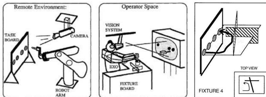
Figure 14: Principle of Virtual Fixtures for trajectory control (adapted from Rosenberg 1992 [29], pp. 15, 20).
