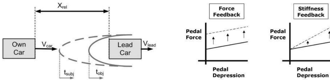
Figure 16: a) Car Following Application of Shared control (adapted from Abbink 2006 [1], pp. 19). b) Schematic representation of force and stiffness feedback mechanism (adapted from Abbink et al. 2008 [2], pp. 7).
