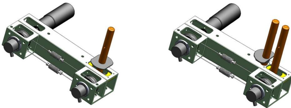
Figure 27: a) View of mechanical design of joystick handle for controlling the winch drum. b) Mechanical design of the grasping joystick for controlling the movement of the clamshells.
