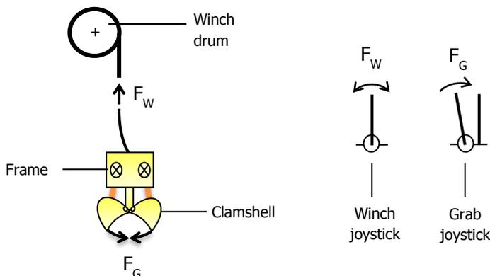
Figure 3: a) Schematic view of control parameters of actuators on slave. b) Schematic view of control parameters of joysticks on master
