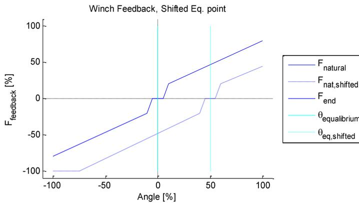
Figure 37: Illustration of the mechanism of shifted equilibrium point of the continuous haptic shared control feedback mechanisms for the winch joystick.
