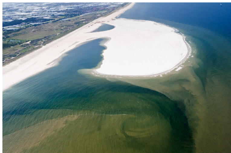
Figure E.2 | The Dutch mega nourishment called the "Sand Engine" (21.5Mm 3 sand) just after construction
