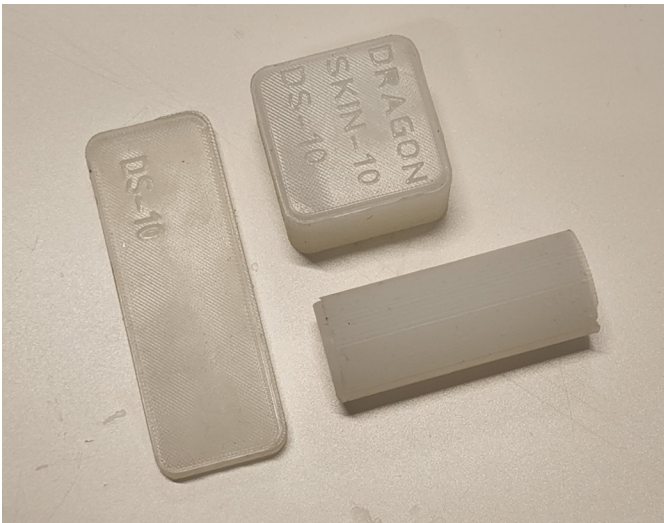
Figure 113. Samples of Dragon Skin 10 silicone. All the silicones tested were in this form.
