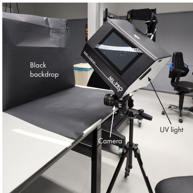
Figure 29. The black backdrop, UV light and camera setup
