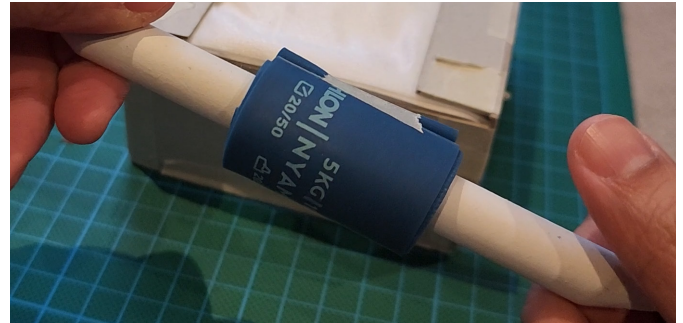
Figure 99. Roller made with natural rubber resistance band (smooth surface)
