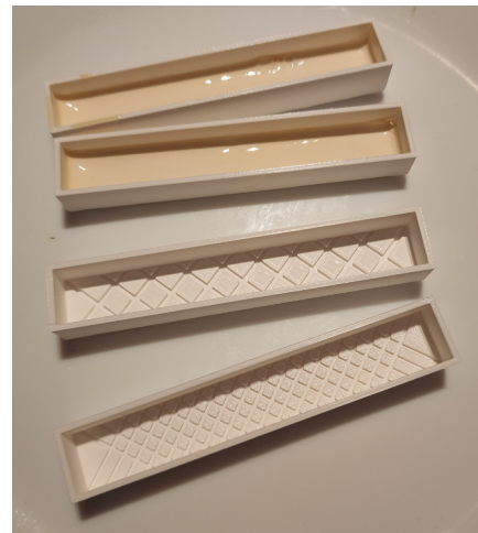
Figure 107. 3D printed molds for natural rubber
