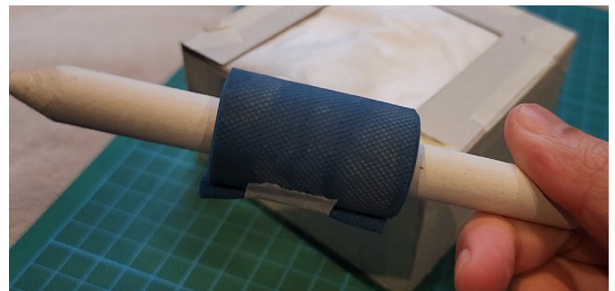
Figure 100. Roller made with natural rubber resistance band (grooved surface)
