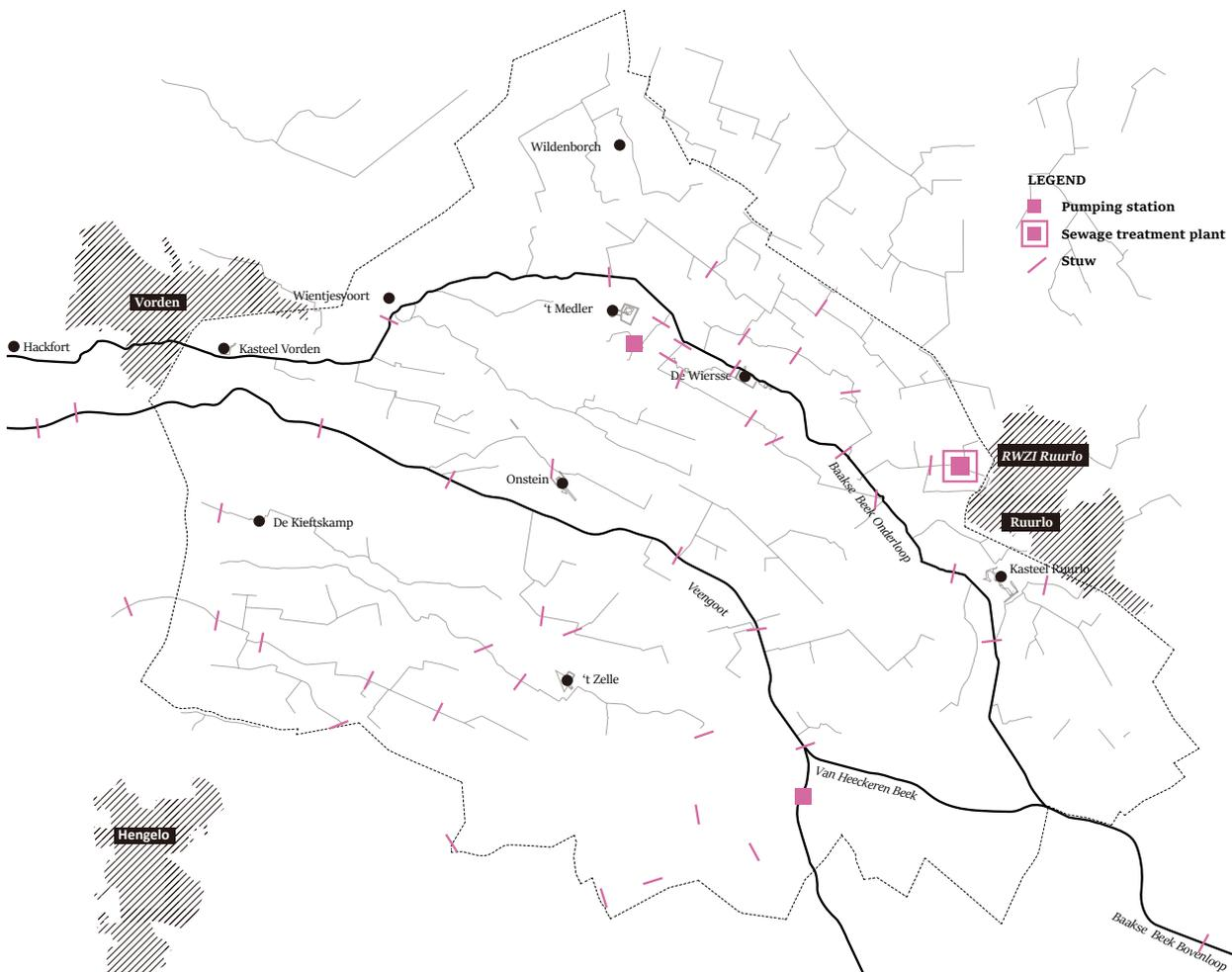
Figure 3.7: A lot of weirs are built on stream for level management. Weir helps retain water in the stream, at the same time slow down the flows and become barriers for migration.
