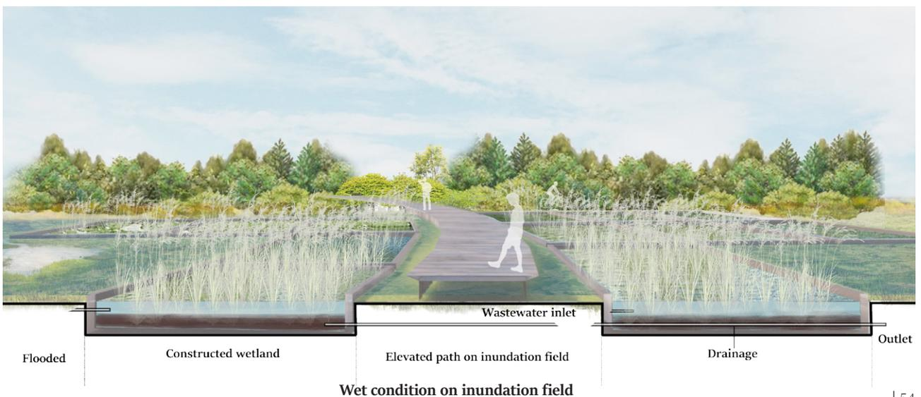
**Figure 5.34: views from the elevated path on an inundation field with constructed wetland tanks installed**
