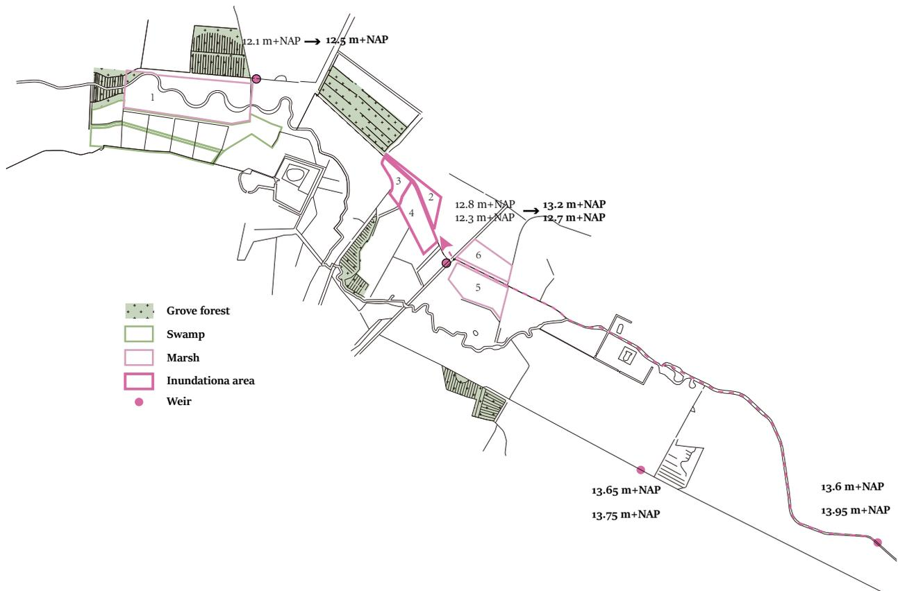
Figure 5.30: wetness restoration measures in water system
