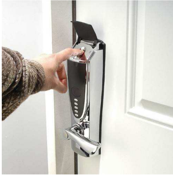
Figure 2-1: An example of a doorlock that uses fingerprint verification as a way to control access. Source: http://walyou.com/biometric-finger-print-door-lock/
