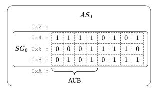
Figure 2.10: Example contents of a segment defined in  $AS_0$  of Figure 2.9b
