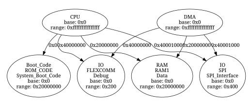
Figure 3.2: AMG graph visualization of an example specification
