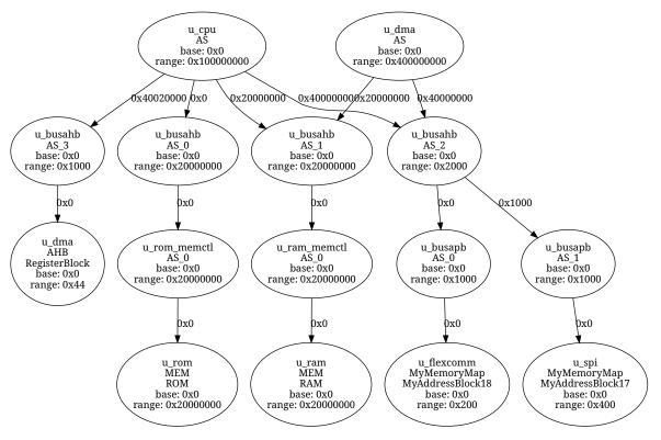
Figure 3.3: AMG graph visualization of an example implementation
