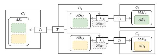
Figure 2.4: Diagram of an IP-XACT construct using a transparent bridge
