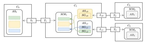
Figure 2.5: Simplified diagram of an IP-XACT construct using an opaque bridge
