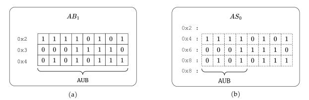
Figure 2.9: Example contents of (a) an addressBlock and (b) an addressSpace
