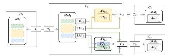
Figure 2.6: Detailed diagram of an IP-XACT construct using an opaque bridge
