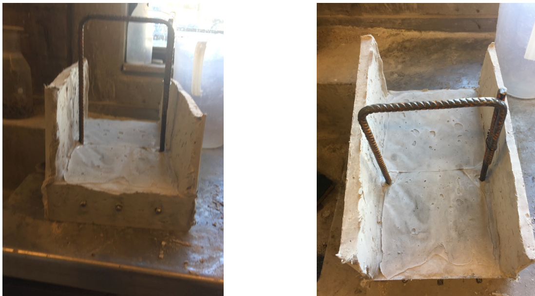
Figure 107 Lab-scale protocol section of SHCC layer with embedded reinforcement system
