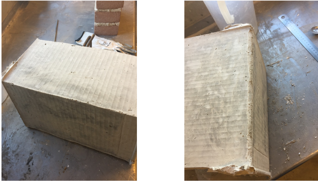
Figure 111 Bottom corners of the element folded after 60 minutes from pouring
