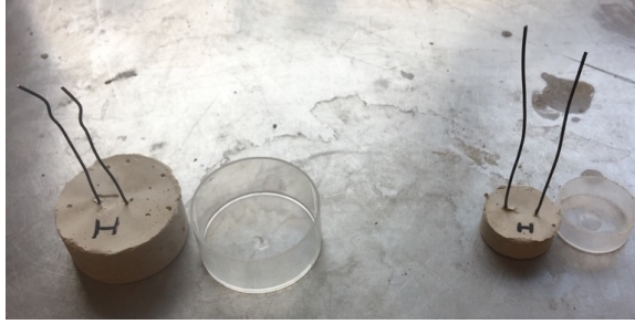
Figure 31 SHCC spacers with height of 31 mm (left) and 11 mm (right)
