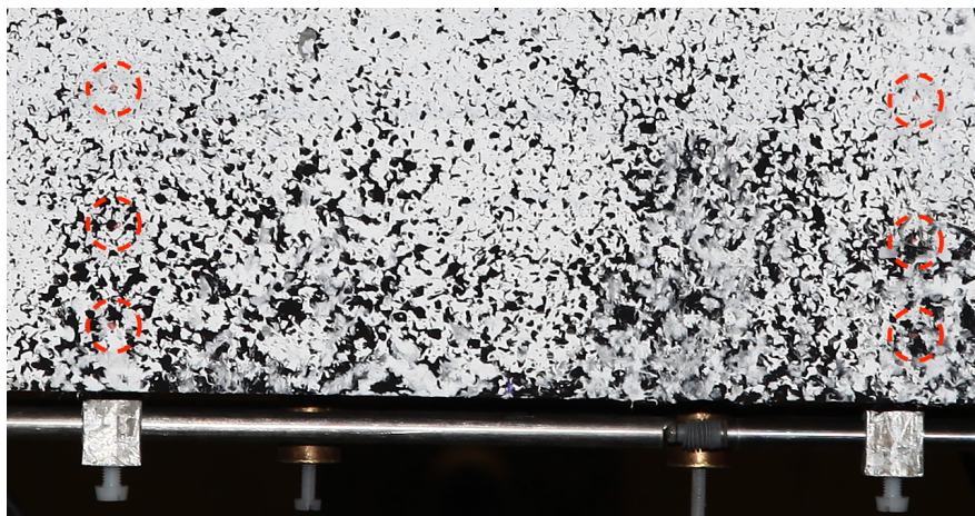
Figure 63 Red dots on the painted surface used during DIC to verify with the LVDT measurements
